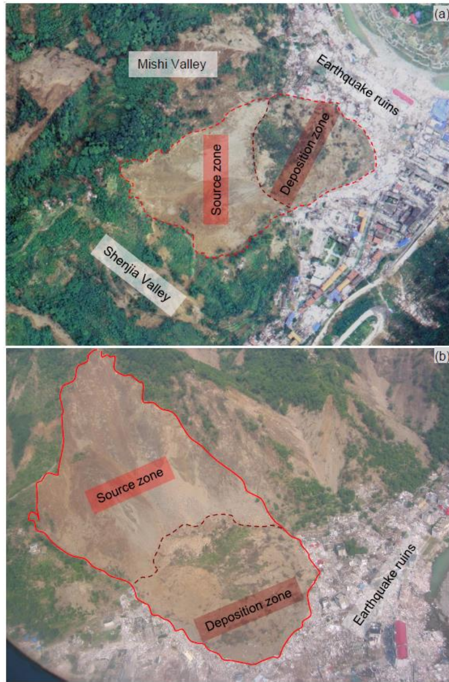
Figure 5 - 1. (a) Airborne remote sensing image of Wangjiayan landslide; (b) Overview of the Wangjiayan landslide.
