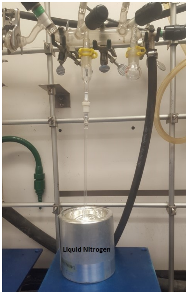
Figure 2.1. Experimental Setup for Condensation of CO in to a J-Young Tube.
