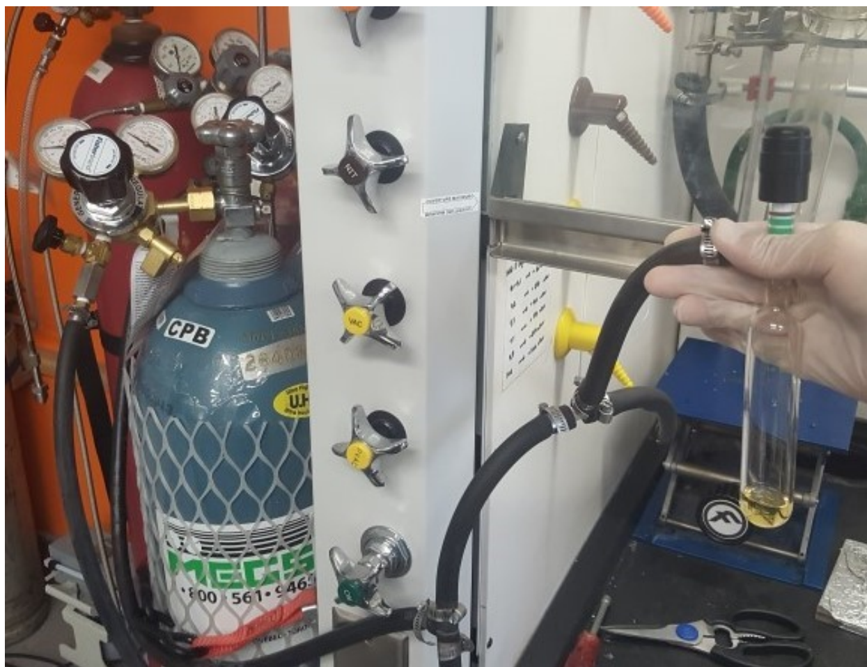
Figure 2.2. Experimental Setup for Carbonylation Reactions (1-4 atm).
