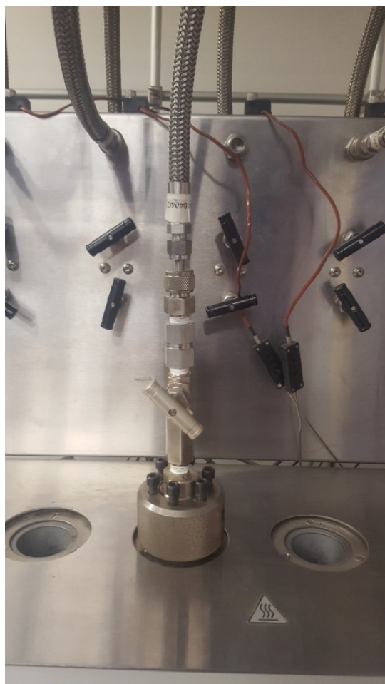
Figure 2.3. Experimental Setup for High Pressure Carbonylation Reactions (5-100 atm).
