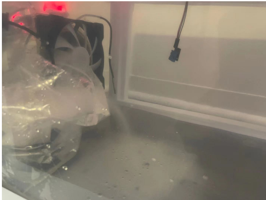
Figure 6: sensor, humidifier and fan of prototype
