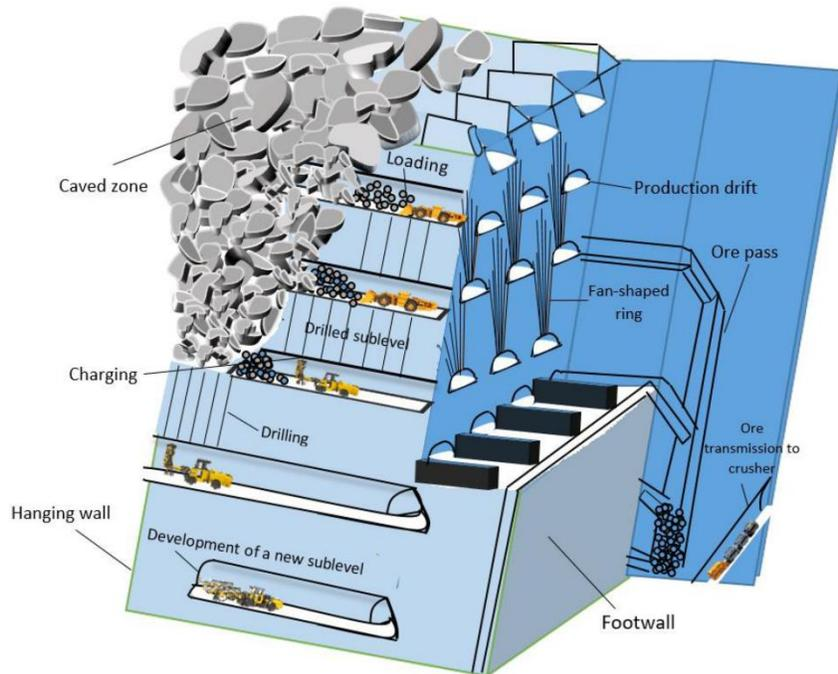
Figure 2-7. Sub-level caving method (Hustrulid & Bullock, 2001)
