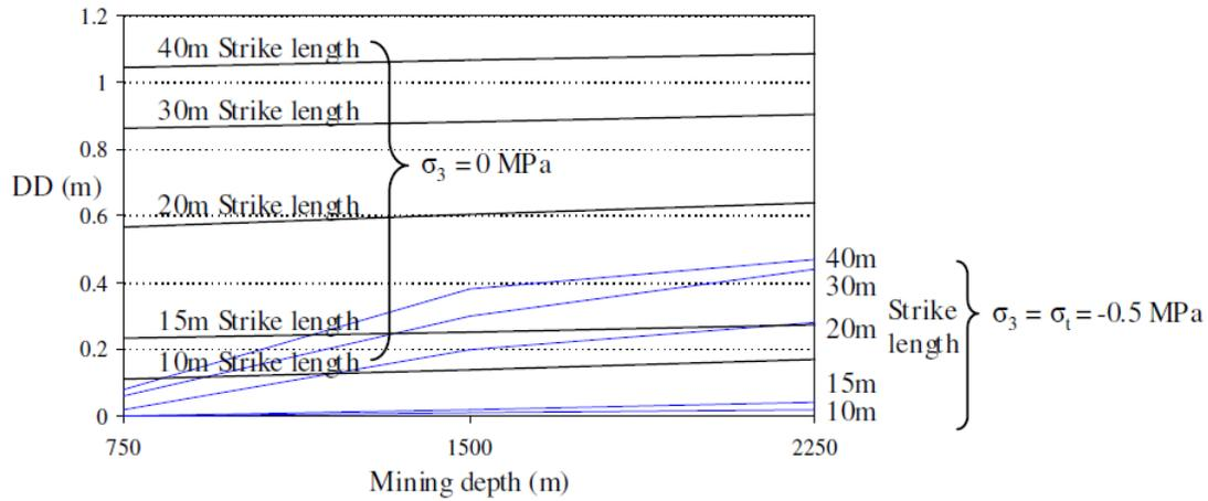
Figure 2-13. Dilution density model according to depth and strike length. Henning et al. (2007)
