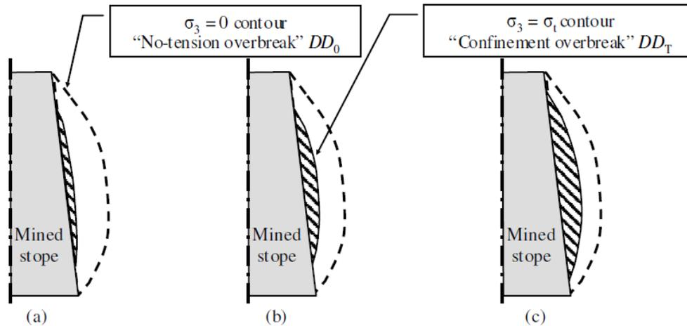
Figure 2-12. Schematic illustration of the influence of mining depth on hanging wall overbreak regimes: (a) shallow depth, (b) moderate depth, and (c) deep. Henning et al. (2007)
