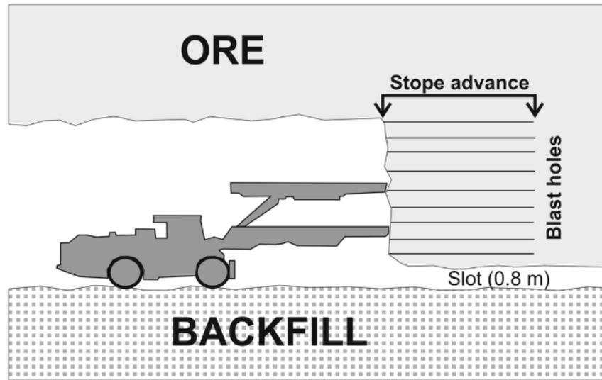
Figure 2-4. Face drilling in the cut-and-fill method (Abzalov, 2016)
