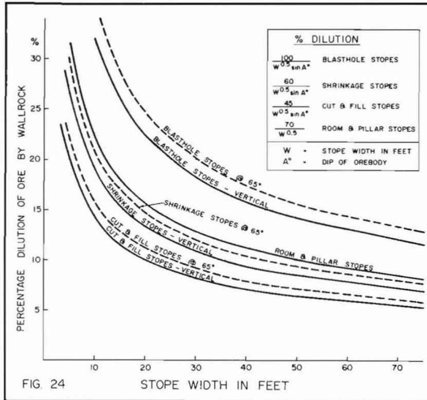
Figure 2-11. O'Hara's plot of stope width against dilution as a function of the mining method and dip angle.
