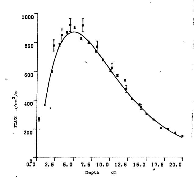
on the outside of the phantom. This is due to neutrons inside the phantom leaking cut. Also, though it may appear that at larger z the experimental points are falling too quickly with respect to the calculated, a single measurement at a depth of 16.3 cm in another run did not drop telow the predicted fluxes. Measurements at greater depths were difficult due to low induced activities in the foils.
