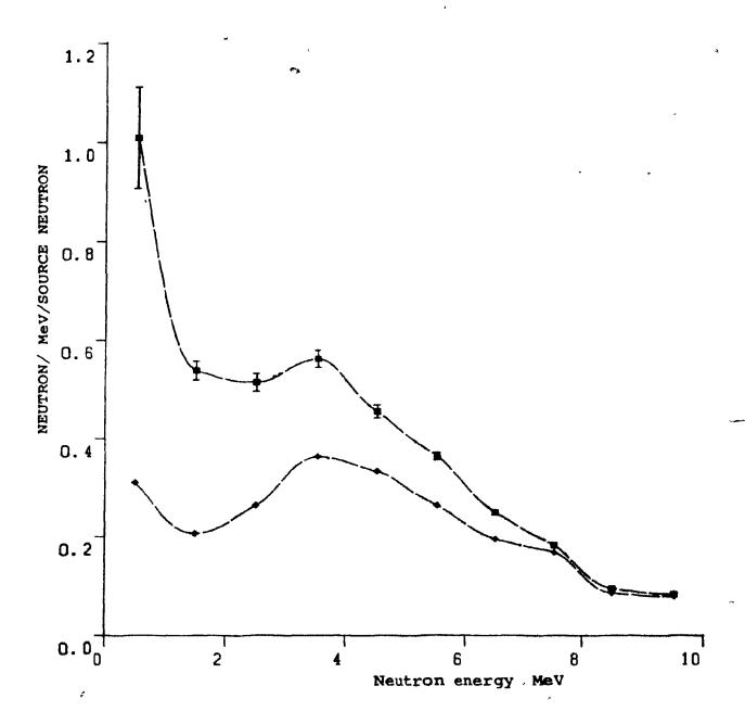
Spectra at two heights in the collimator due to an AmBe source. Curve is eyequide only.
