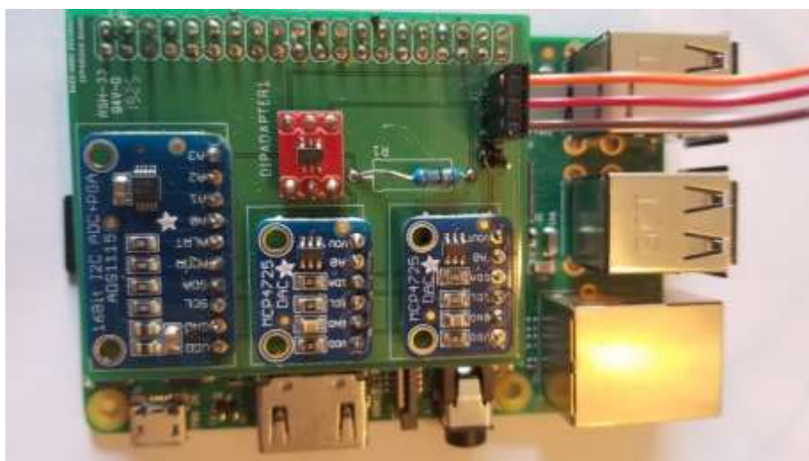
Fig. 3.13: Interrogation circuit with a ribbon cable that terminates at the graphene ISFET holder.
