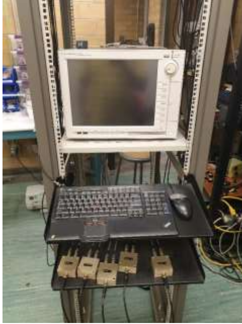
Fig. 2.1: The Agilent Technologies B1500A SPA that was used for measuring I_{ds} versus time as the concentration of the analyte is increased.
