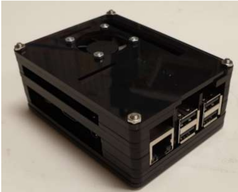
Fig. 3.7: (a) A picture of an SBC board enclosed in its case [32]. (b) A picture of the interrogation circuit enclosed in the case we created by combining the Raspberry Pi 3 Model B Smraza Compatible cases [32].
