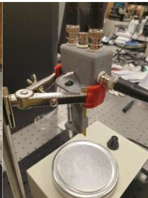
Fig. 2.3: The sensor holder with the ISFET sensor and reference electrode (a) front view (b) side view.
