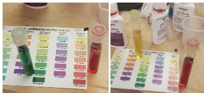
Figure 4.3 Measurement of ammonia and nitrates using an API test kit of fresh manure extract (left) and biojuice once nitrification is complete (right).
