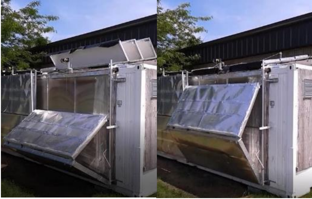
Figure 2.5 Opening (left) and closing (right) of the CING insulating panels
