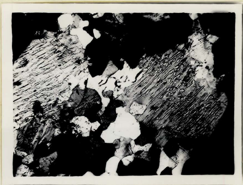
Plate No. 51. Showing microperthite with good rods of albite. A small crystal showing an indistinct vermicular texture may be seen between the two large crystals. Hornblende syenite. Nicols crossed, X 32.
