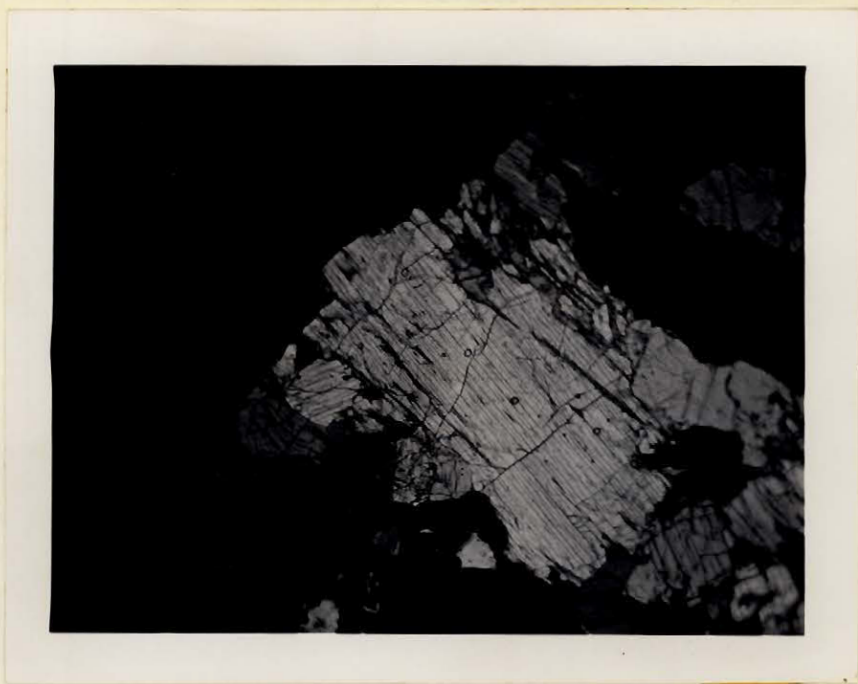
Plate No. 49. Large crystal of hypersthene in coarse grained porphyroblastic hypersthene-augite-hornblende rock. (See Plate No. 15) Showing good 010 cleavage. Nicols crossed, X 20.
