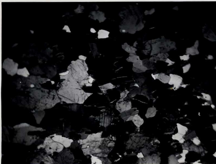
Plate No. 42. Biotite gneiss from Lac des Montagnes. Note the slight reaction rims around the biotite in the centre of the section, and the bent albite twinning. This section shows weak albitization. Nicols uncrossed, X 20.
