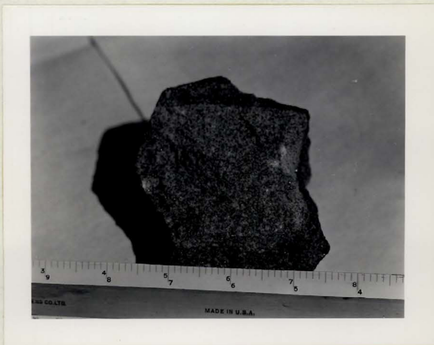
Plate No. 24. "Granitized" looking biotite garnet gneiss showing depth of weathering.
