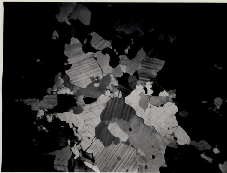
Plate No. 48. Medium grained granoblastic matrix surrounding clusters shown in Plate No. 47. Note abundant twinning which is normally scarce in the rocks of the area. Nicols crossed, X 20.
