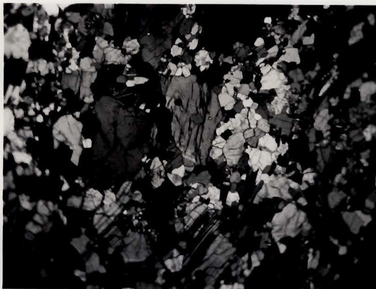
Plate No. 37. Garnet gneiss with weak preferred orientation, showing some fracturing of the larger feldspar crystals. The smaller crystals may be of cataclastic origin. Nicols crossed, X 20.
