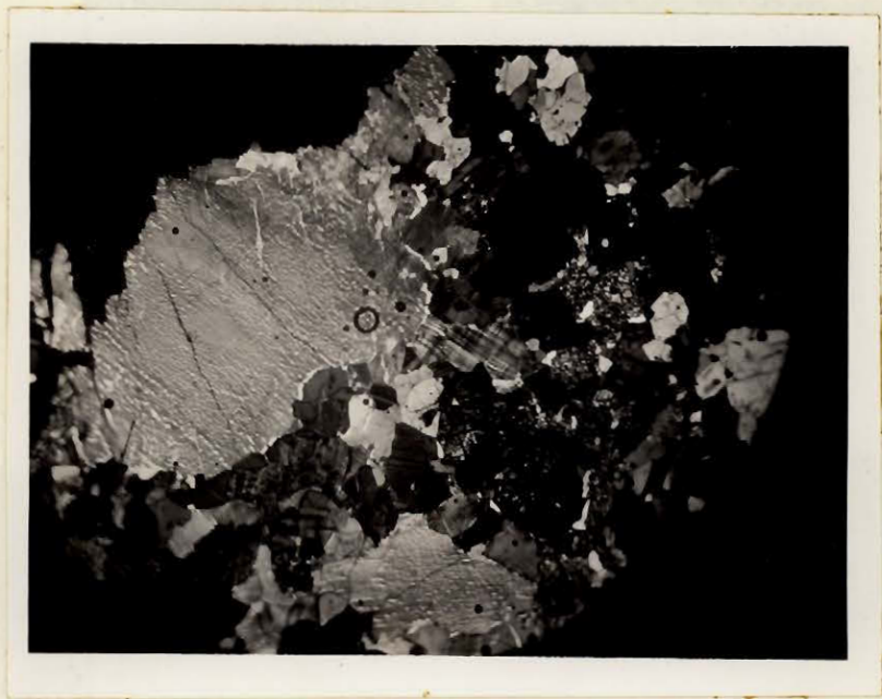
Plate No. 50. Microperthite in hornblende syenite. Note albite filling fractures and apparently starting to replace the margins of the large crystal. The small fresh crystal of microcline is partly surrounded by a resorbed pyroxene that could be either hypersthene or aegirine-augite.
