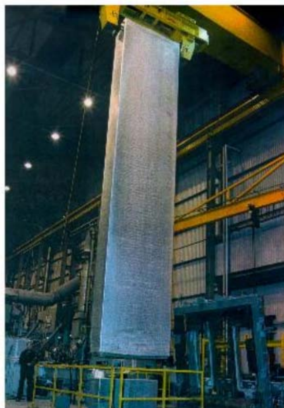
Figure 1.4: A rolling ingot is removed from casting pit at the end of the DC casting process [1].
