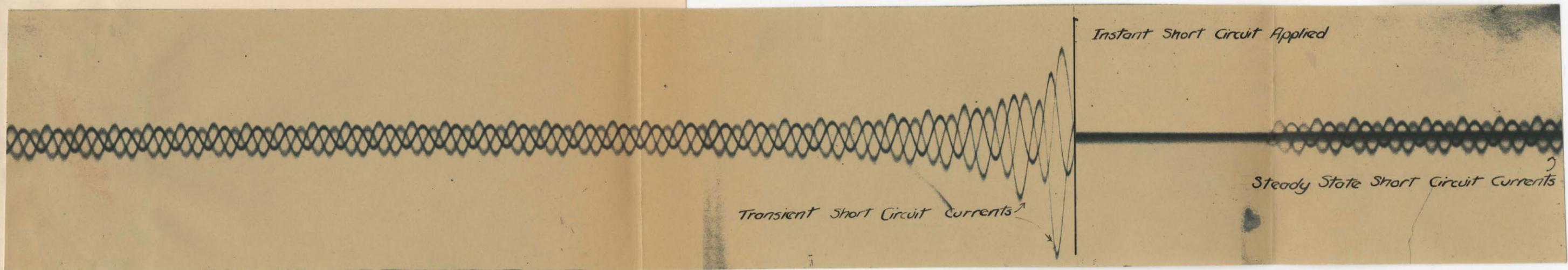
OSCILLOGRAM OF A THREE PHASE SHORT CIRCUIT
