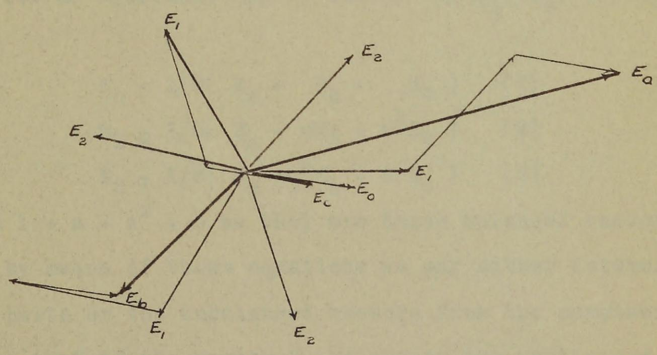
Since these systems are equivalent to a single unbalanced system, if  $E_a$ ,  $E_b$ , and  $E_c$  are the unbalanced vectors then;
