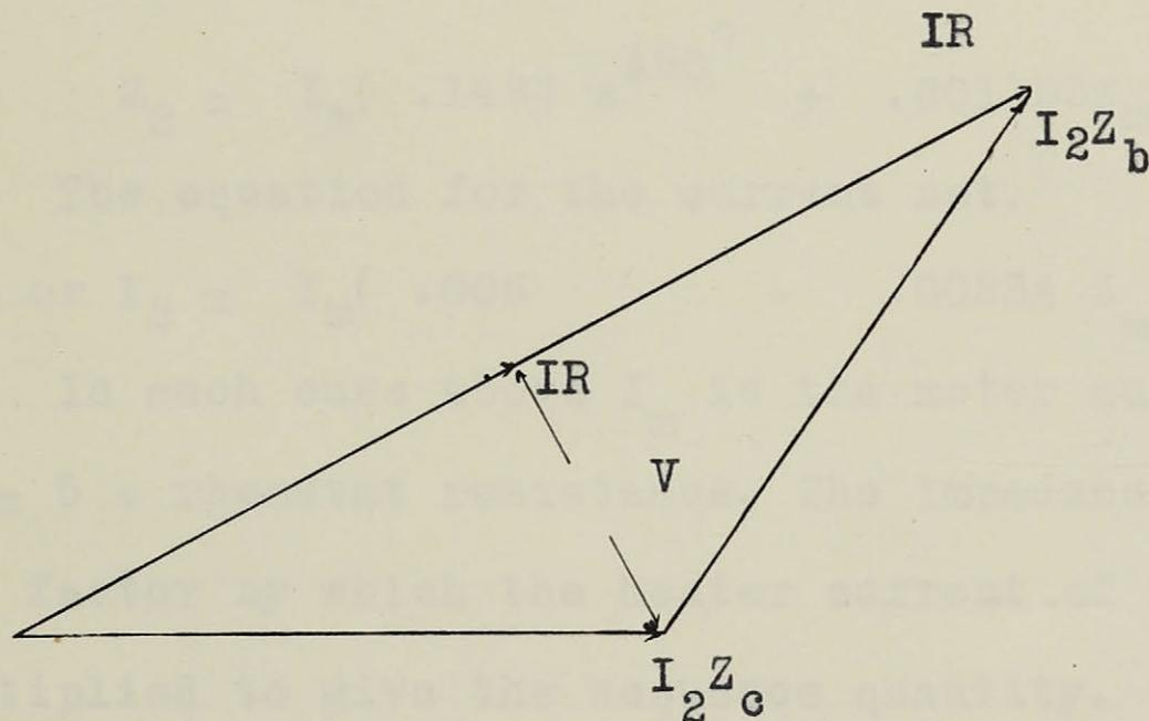
The resistance of  $Z_b$  was adjusted until the two voltages had this relation to each other. Approximately 10 amps were passed through branch  $Z_b - Z_c$  giving a drop of about 30 volts.
