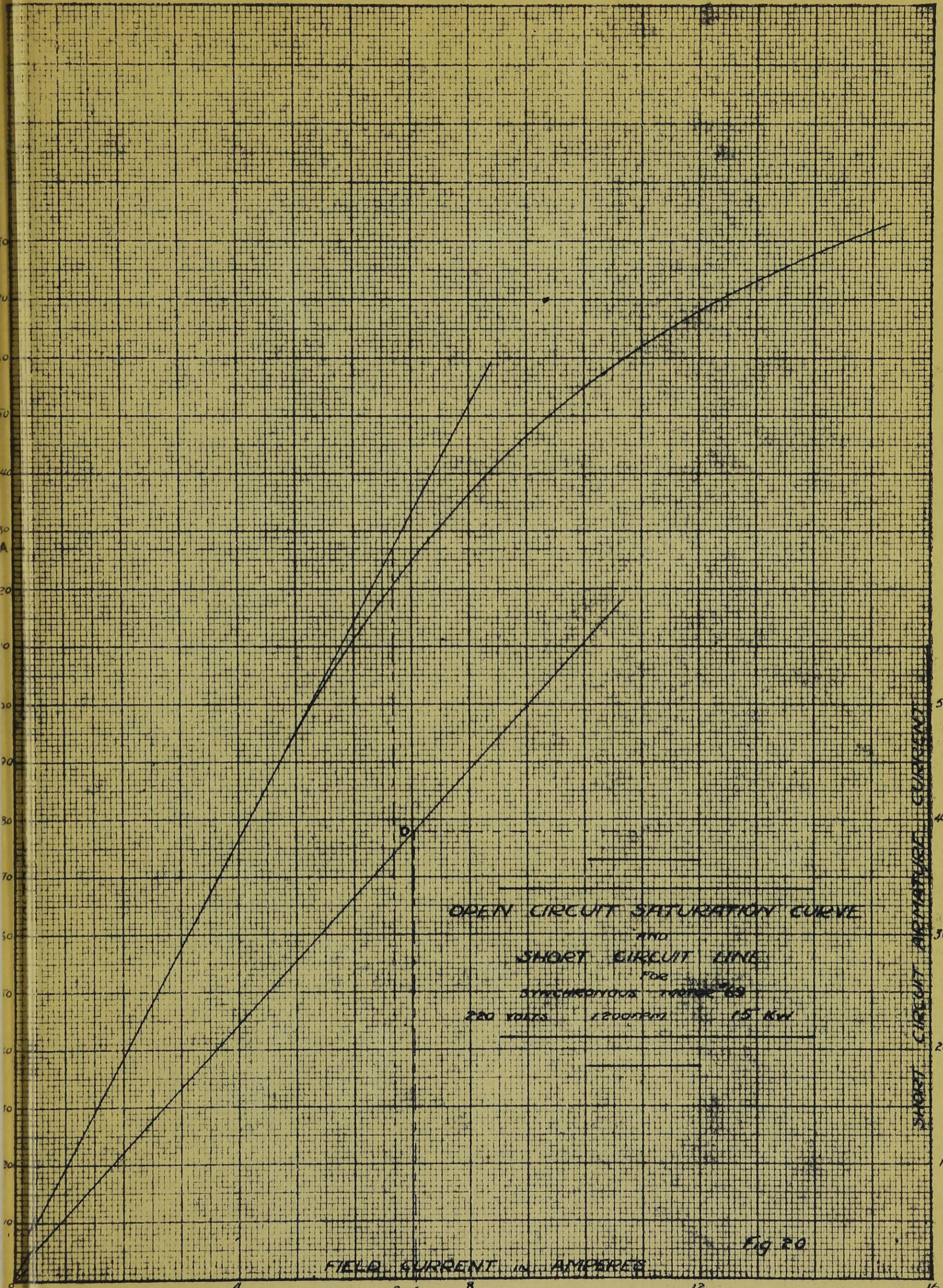
OPEN CIRCUIT SATURATION CURVE
