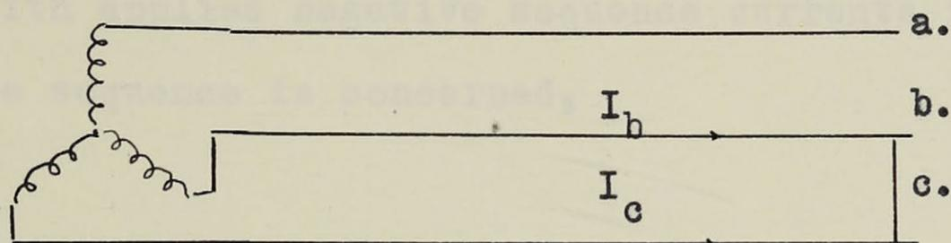
Consider a short circuit between phases b and c
