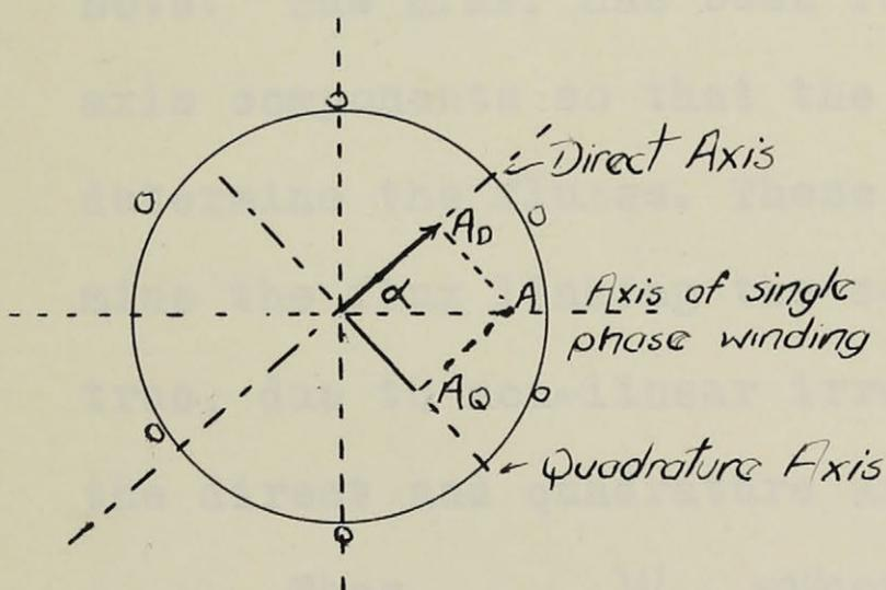
Referring to the figure to the left which shows a three phase armature winding with single phase applied voltage:
