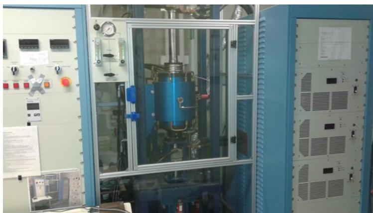
Figure 3.5 Thermal Technology LLC 10-3 SPS apparatus
