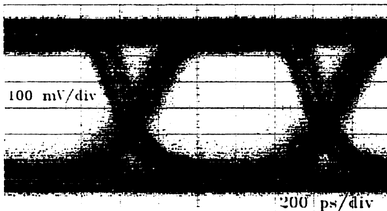
Figure 5.5. Eye pattern at 1Gb/s from the optical source used to test the receiver
