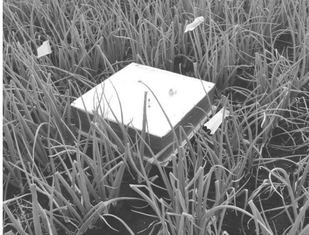
**Figure 19: A static non-steady state chamber installed for gas sampling**
