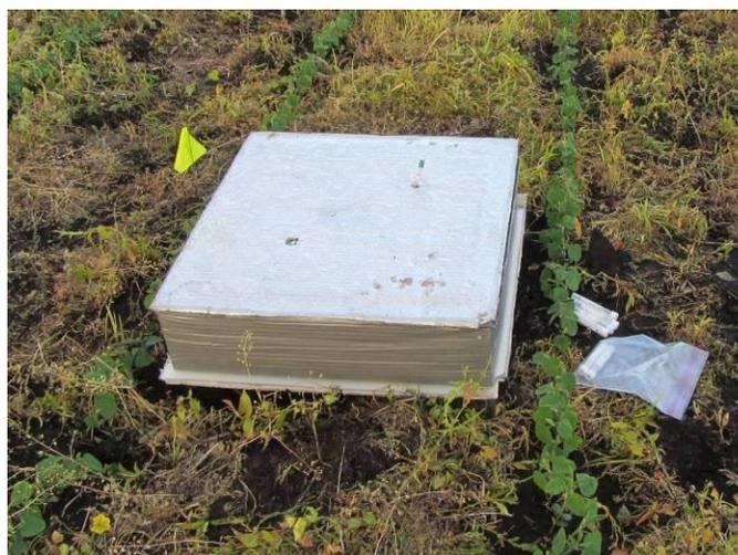
**Figure 26: Non-steady state chamber design deployed between soybean crop, covered with aluminum sheet to minimized the effect direct thermal from the sun.**
