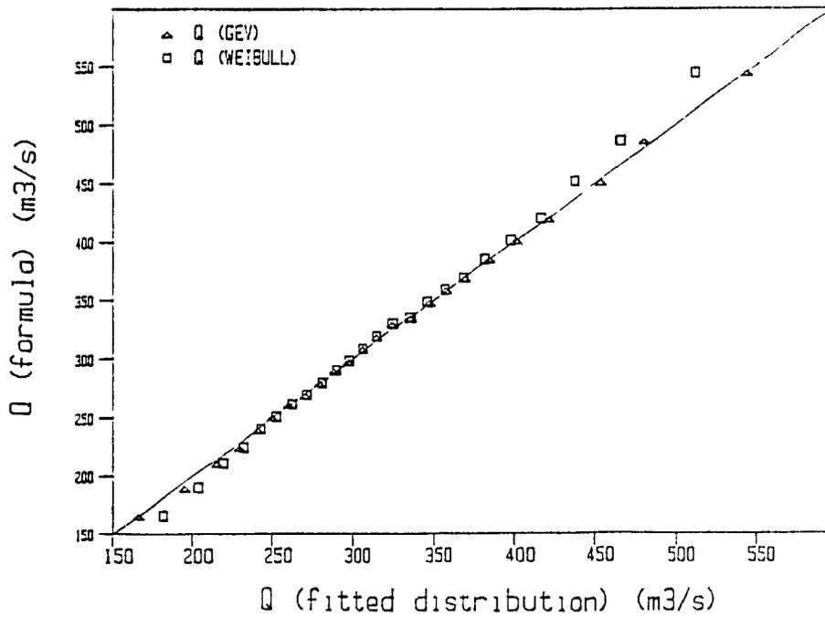
Figure 6.3 Quantile-quantile plot of P3, GEV and Weibull formulas
