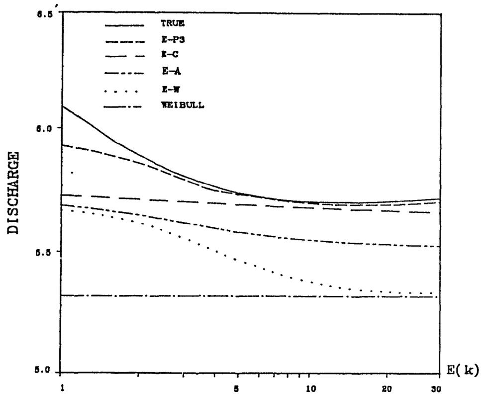
Figure 5.10 Bias in discharge for P3 distribution,  $\gamma = 1$ .
