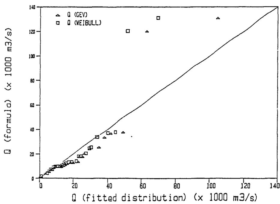
Figure 6.4 Quantile-quantile plot of P3, GEV and Weibull formulas (Huangbizhuang River,  $C_{su} = 3.0, N = 25$ ).
