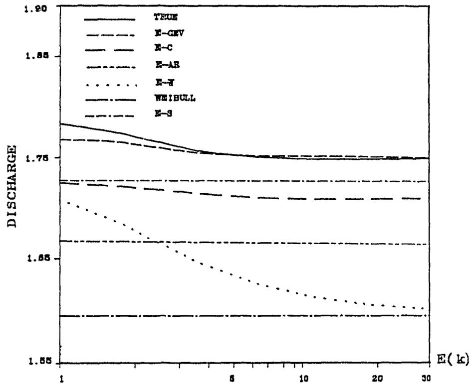
Figure 5.12 Bias in discharge for EV2 distribution,  $\gamma = 2$ .
