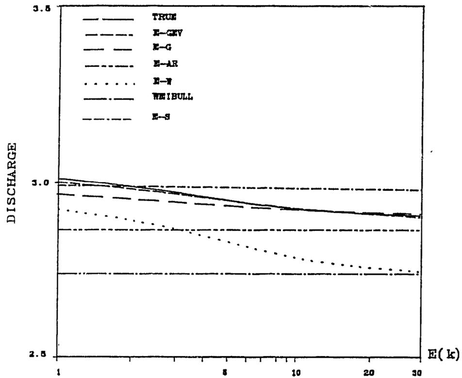
Figure 5.11 Bias in discharge for EV1 distribution,  $\gamma = 1.139$ .
