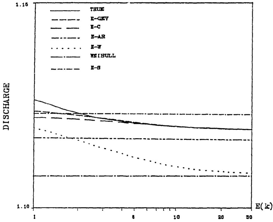
Figure 5.13 Bias in discharge for EV3 distribution,  $\gamma = 1$ .
