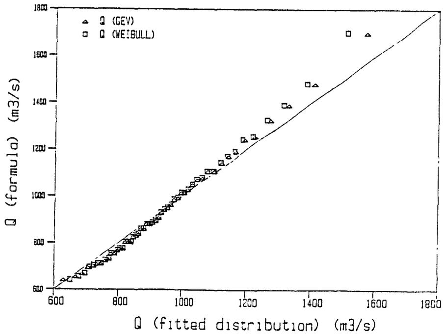
Figure 6.2 Quantile-quantile plot of P3, GEV and Weibull formulas
