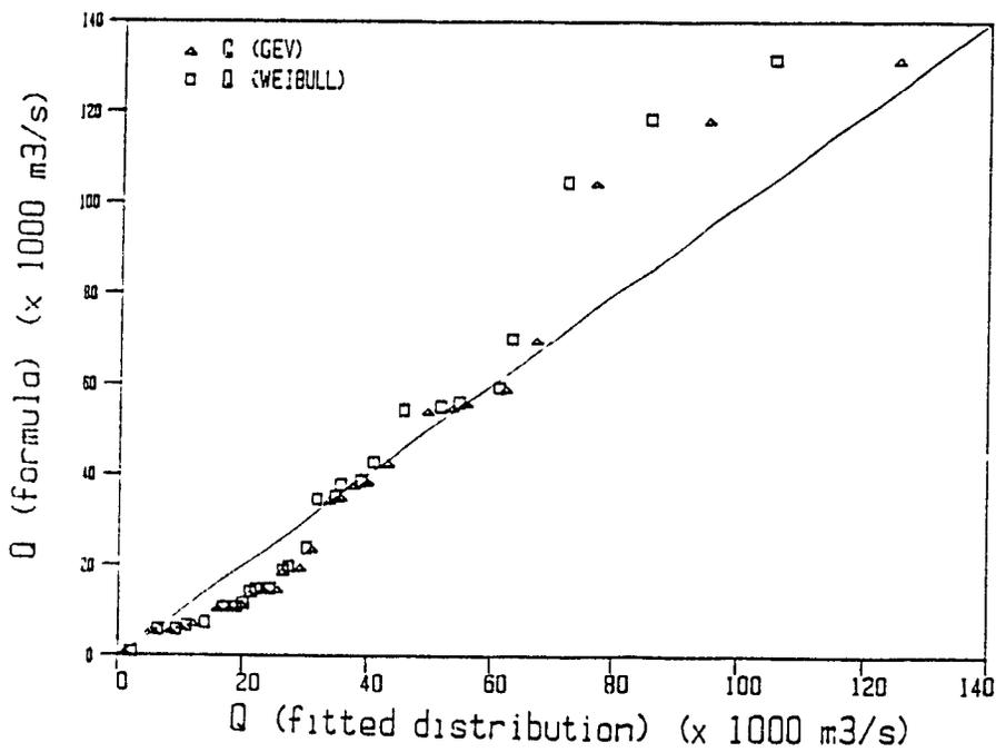
Figure 6.5 Quantile-quantile plot of P3, GEV and Weibull formulas
