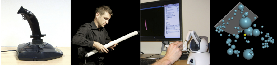
Fig. 1 Examples of some of the types of devices we wish to flexibly connect to media synthesizers. Clockwise from top-left: commercial computer input devices such as joysticks, “novel” musical instruments such as the T-Stick [18] (photo: Vanessa Yaremchuk), force-feedback/haptic devices, and systems for modelling virtual physical dynamics such as DIMPLE [28].
