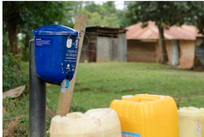
Figure 8: Chlorine dispenser and jerry can containers © Evidence Action
