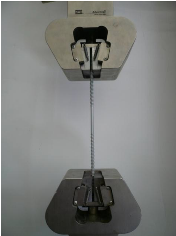
Figure 4-45 Picture of screw tensile test setup (Prat-Vincent 2011)
