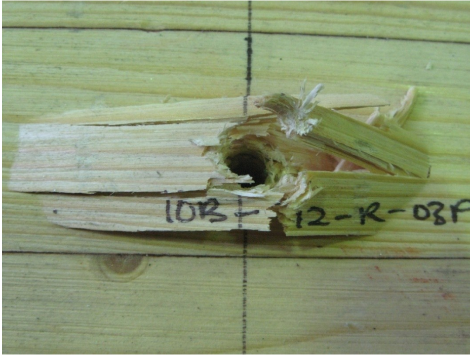
Figure 4-2 Detail showing Withdrawal failure
