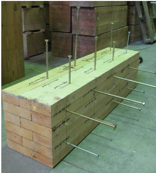
Figure 3-11 Glulam member with markings and installed screws prior to testing
