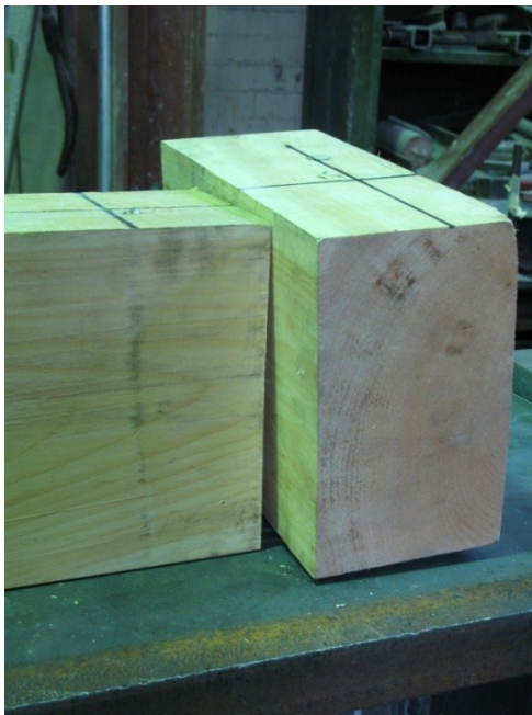
Figure 5-2 Gaps at joints of the dried cross screw connection assemblage
