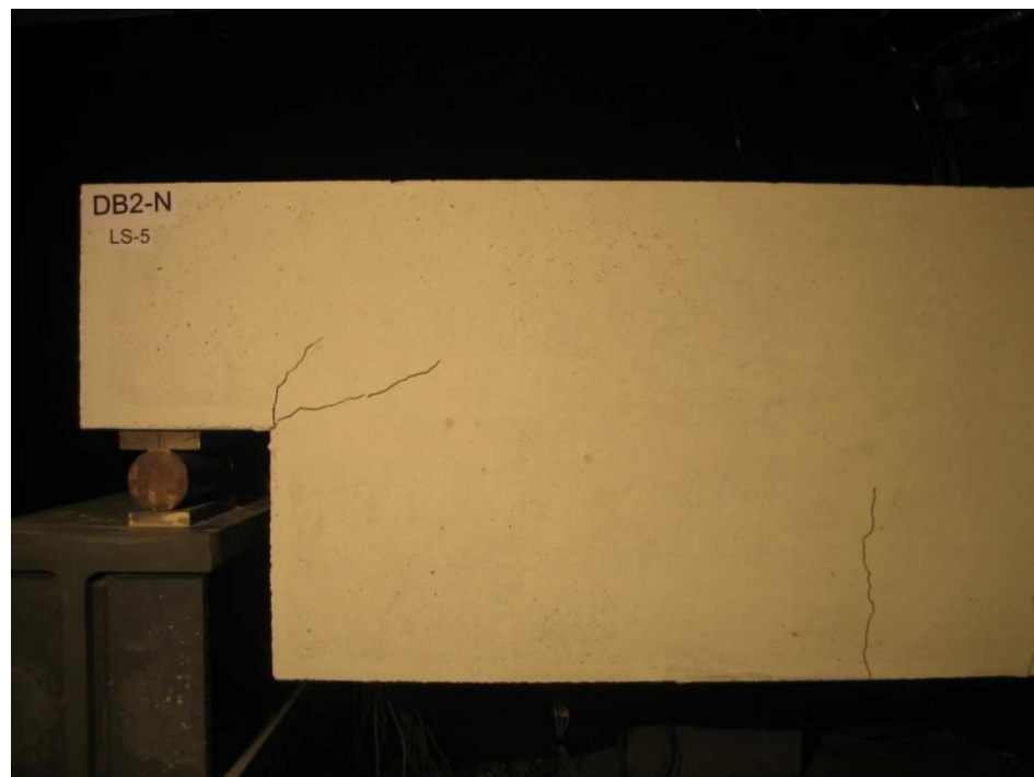
Figure 3.35 Photo of crack pattern at LS-5 for DB2-N
