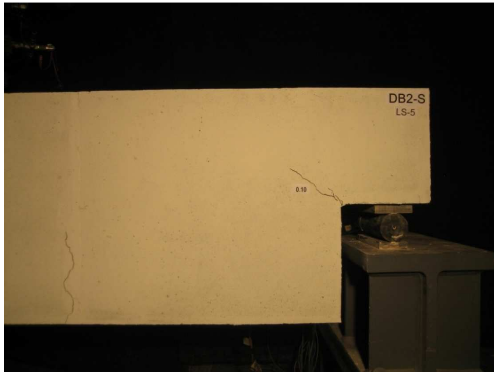
Figure 3.267 Photo of crack pattern at LS-5 for DB2-S
