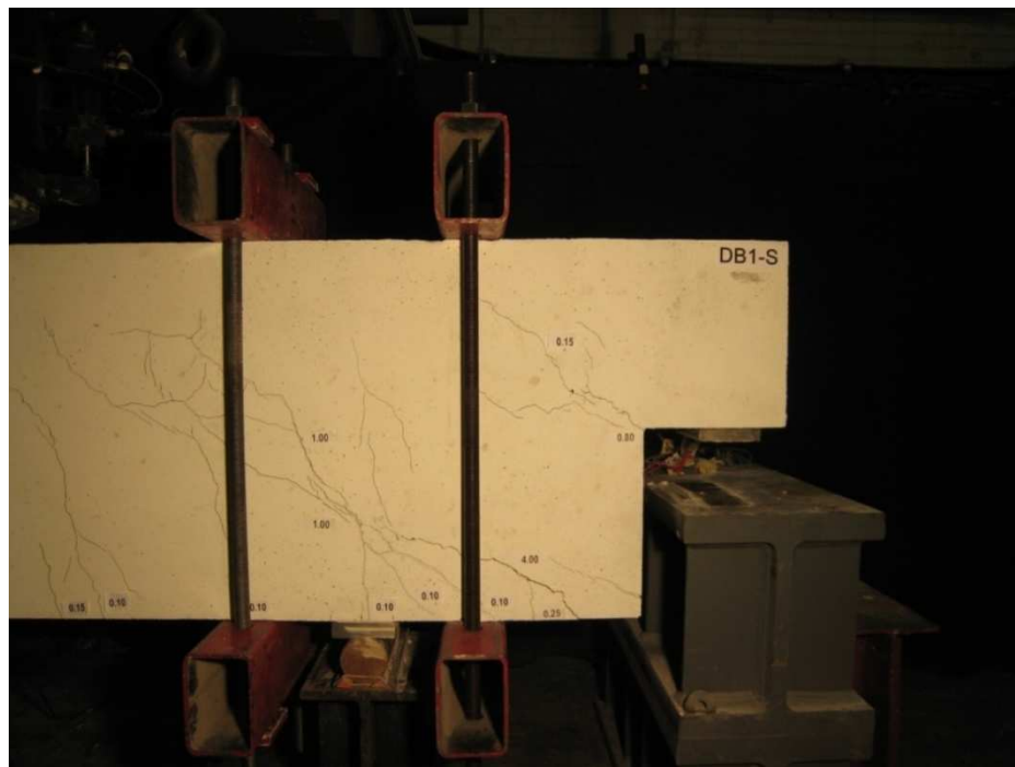
Figure 2.26 Retrofit of DB1 at south end
