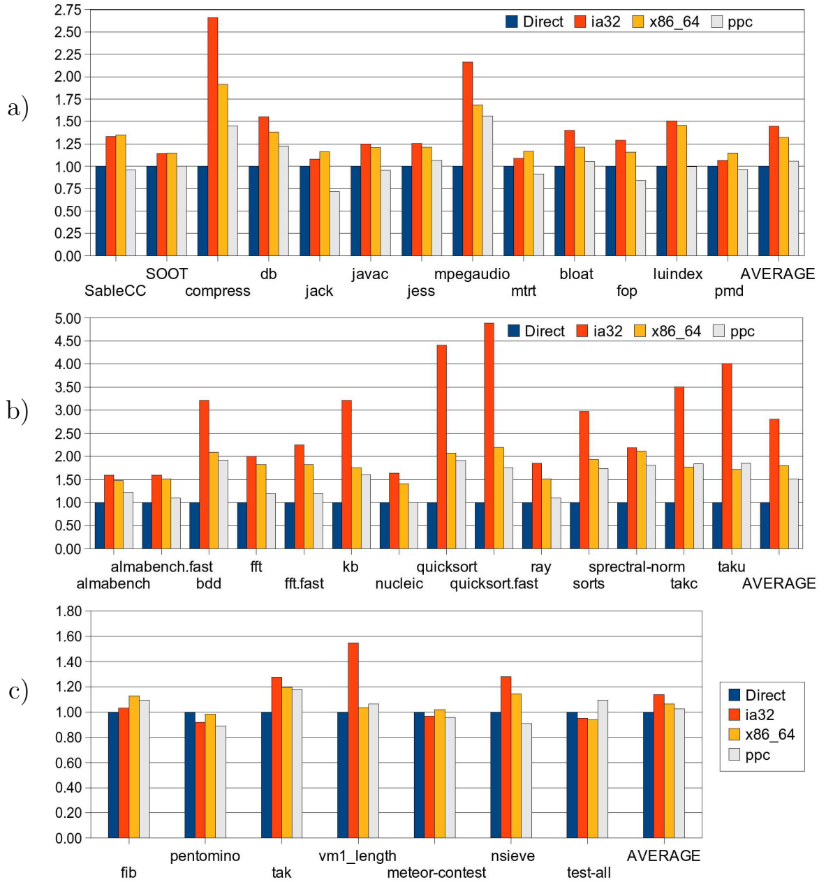
Figure 5.2: Performance (speedup) results for a) SableVM (Java), b) OCaml, and c) Yarb (Ruby). Note in this figure we measured the overall VM performance, as opposed to other results in this chapter that measure VM behavior only within the interpreter function.
