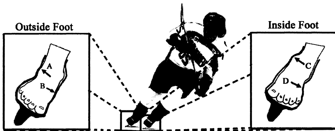
Figure 15: Arrows indicate which sensor, compared to the sensor on the opposite side of the foot, demonstrates the highest amounts of pressure. On the outside foot the lateral maleolus (A), medial calcaneus (B) and on the inside foot the medial maleolus (C), lateral calcaneus (D) displayed the highest pressures which demonstrates a levering effect of the ankle and foot in the skate boot.
