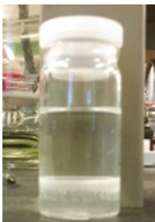
Figure 20: Picture of a typical catalytic test for the epoxidation of methyl oleate. The catalyst ( [\text{DP}^{2+}]_3[\text{PPW}^{3-}]_2 ) floats between the organic phase (top) and the aqueous phase (bottom).
