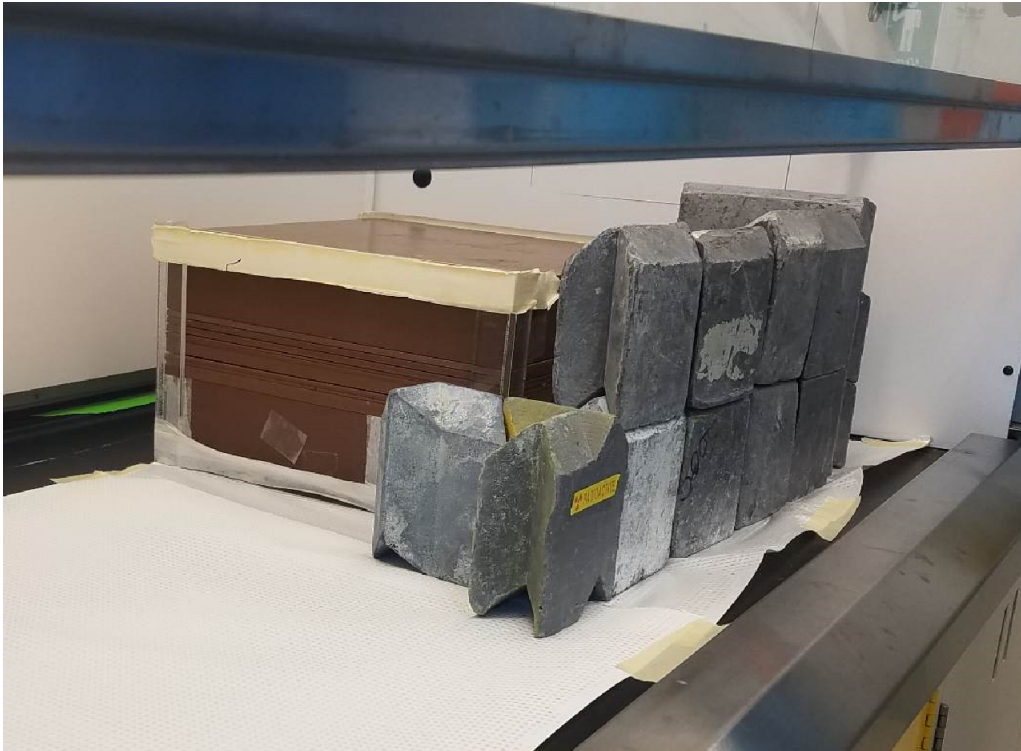
Figure 3.2: Measurement setup for film measurements. Solid water phantom is located behind lead bricks for radiation safety. The films were placed and centered on each slab.
