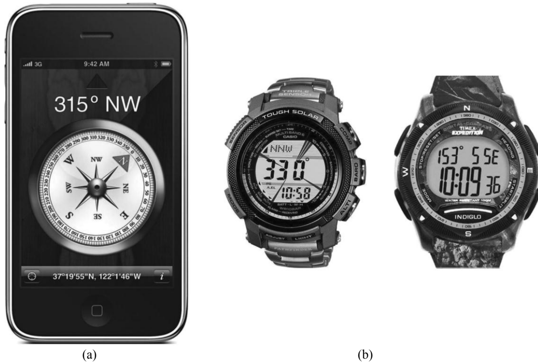
Figure 4.17: Examples of e-compasses integrated in: (a) cell phone <Apple>, (b) watches <left: Casio, right: Timex> [5].
