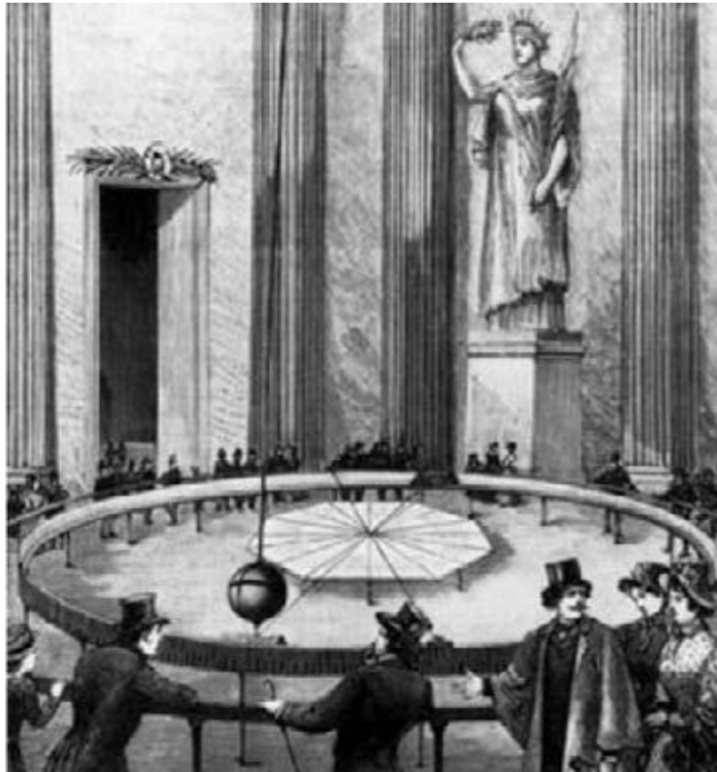
Figure 2.2: The Foucault pendulum, invented by Jean Bernard Léon Foucault in 1851 as an experiment to demonstrate the rotation of the earth. The swinging direction of the pendulum rotates with time at a rate proportional to the sine of the latitude, due to earth's rotation [2].
