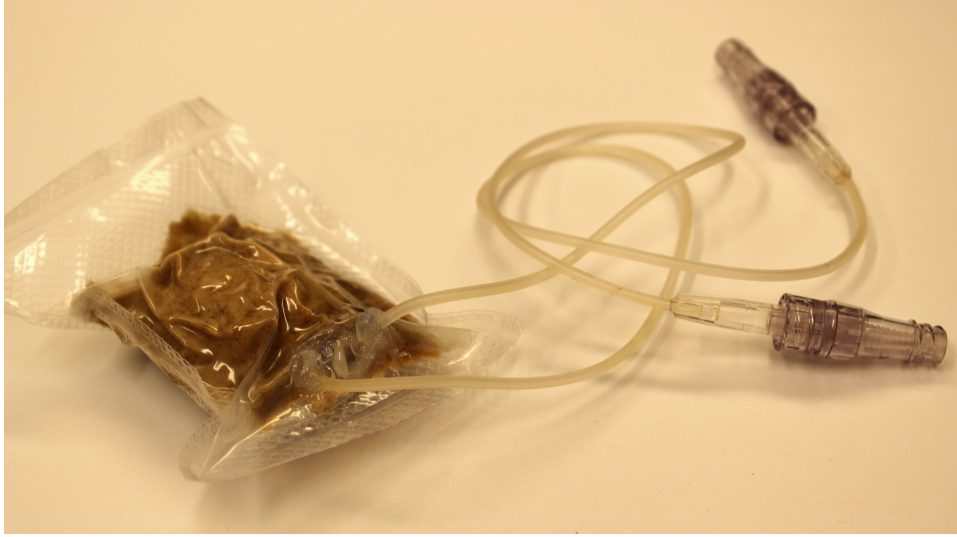
Figure 5–4: Photo of the synthetic tumor consisting of multiple vacuum sealed compartments.
