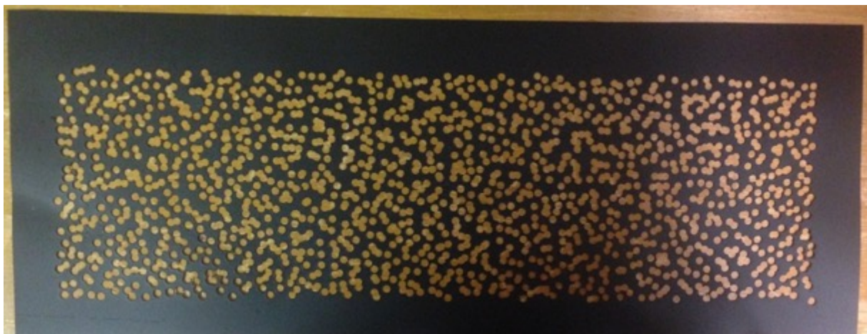
Figure 4.5: Speckle pattern stencil.
