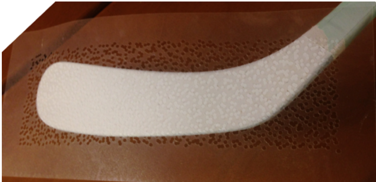
Figure 4.6: Blade with base coat and stencil prior to speckle painting.
