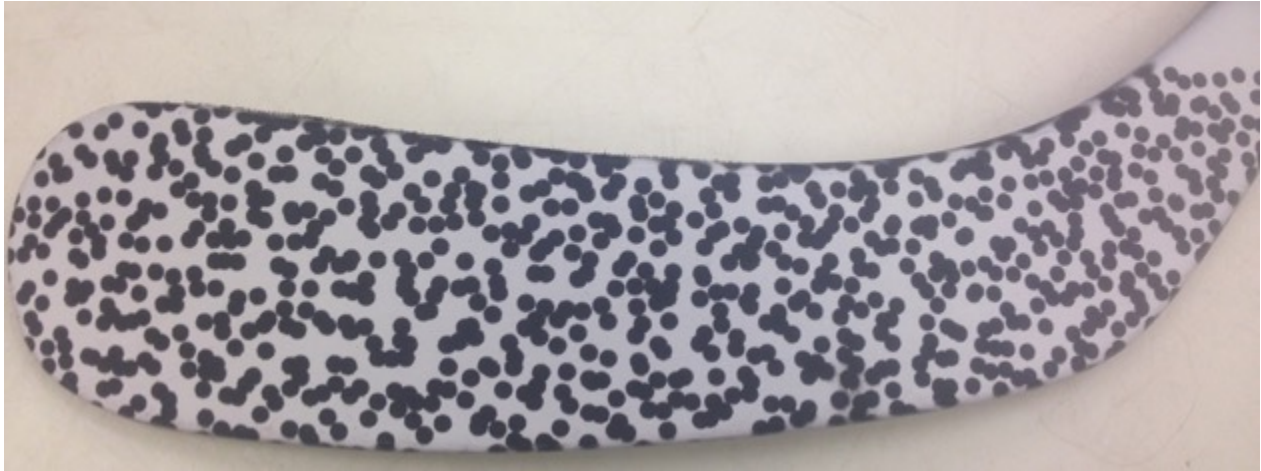
Figure 4.7: Final blade with speckle pattern.
