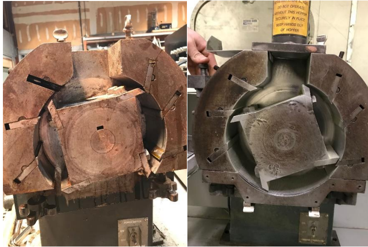
FIGURE 15. ROTOR PLACE INCORRECTLY IN LEFT PHOTO.
