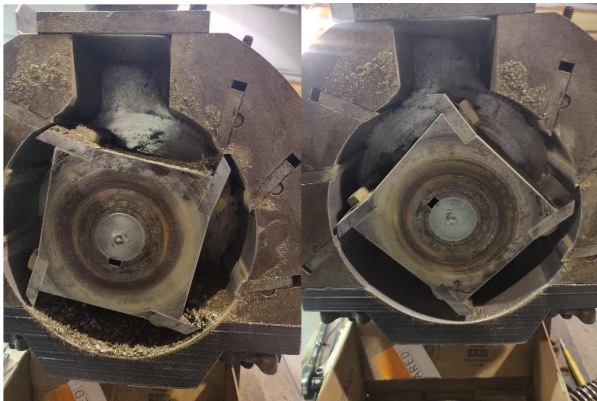
FIGURE 21. FIGURE ON LEFT IS AFTER GRINDING, FIGURE ON RIGHT IS AFTER CLEANING CYCLE
