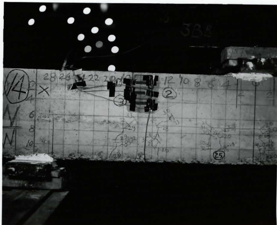
Plate 17 - Beam 14, Span with First Diagonal Crack (34 kips), (West).
