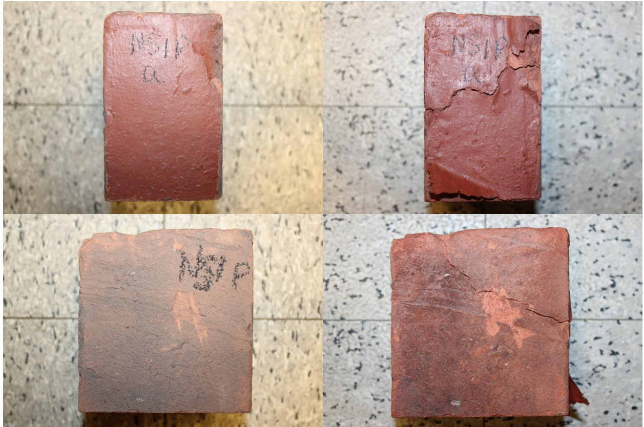
Figure 3.5. BERRi-NS-IP before and after the freeze-thaw test
