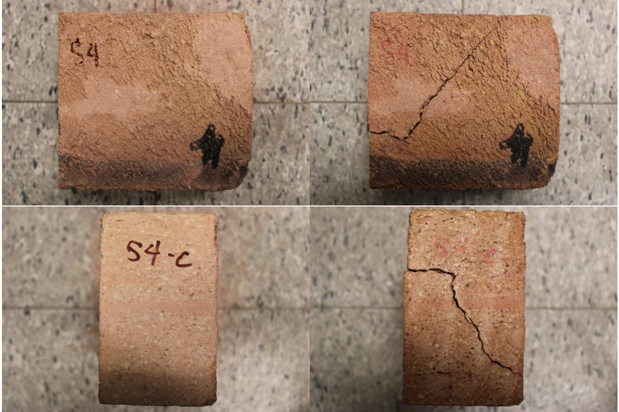
Figure 3.1. ORANGE-4 before and after the freeze-thaw test
