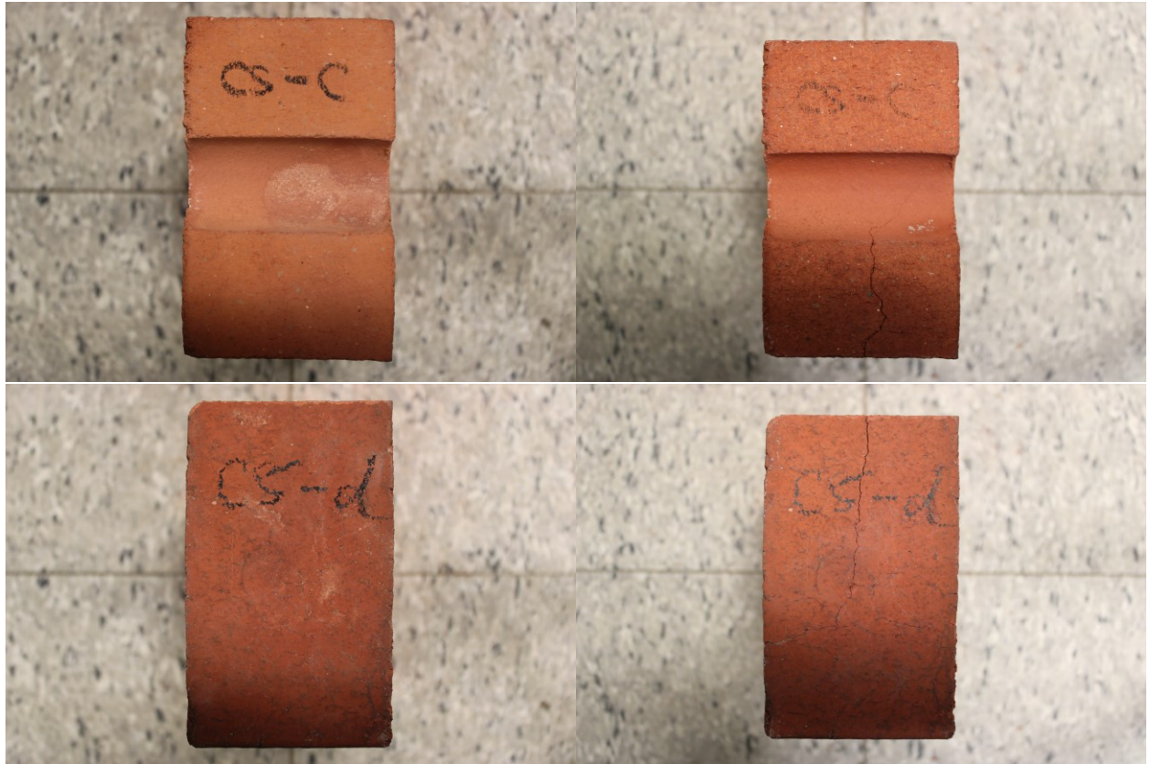
Figure 3.3. CORED-5 before and after the freeze-thaw test
