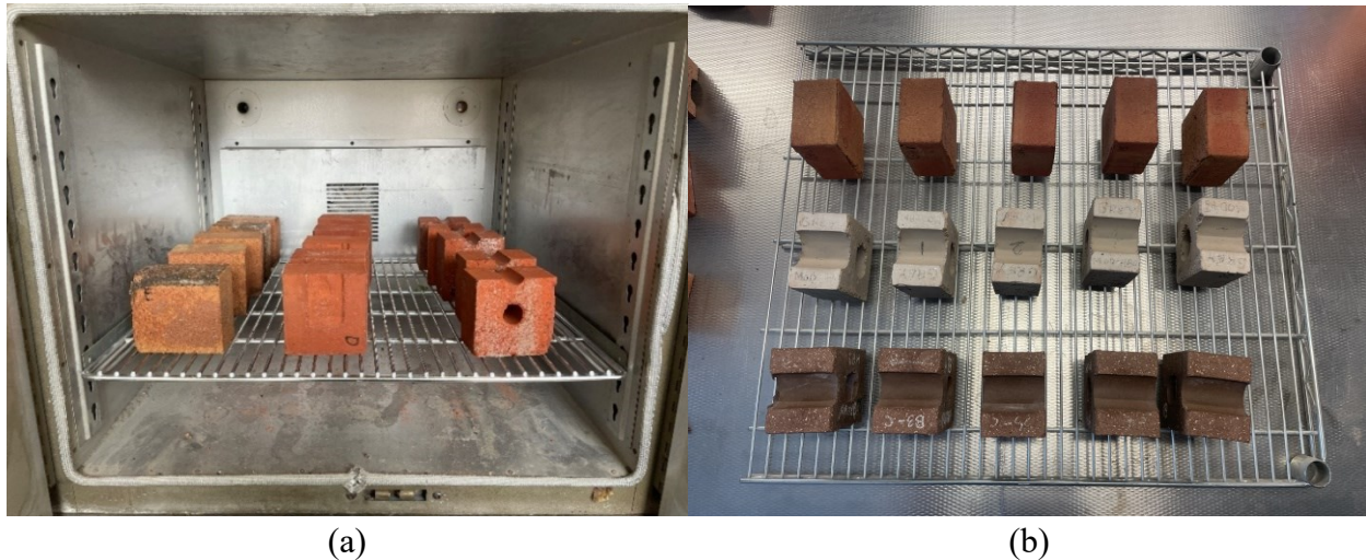
Figure 2.5. (a) Half-bricks drying in the oven at 115°C; (b) half-bricks cooling on a metal rack
