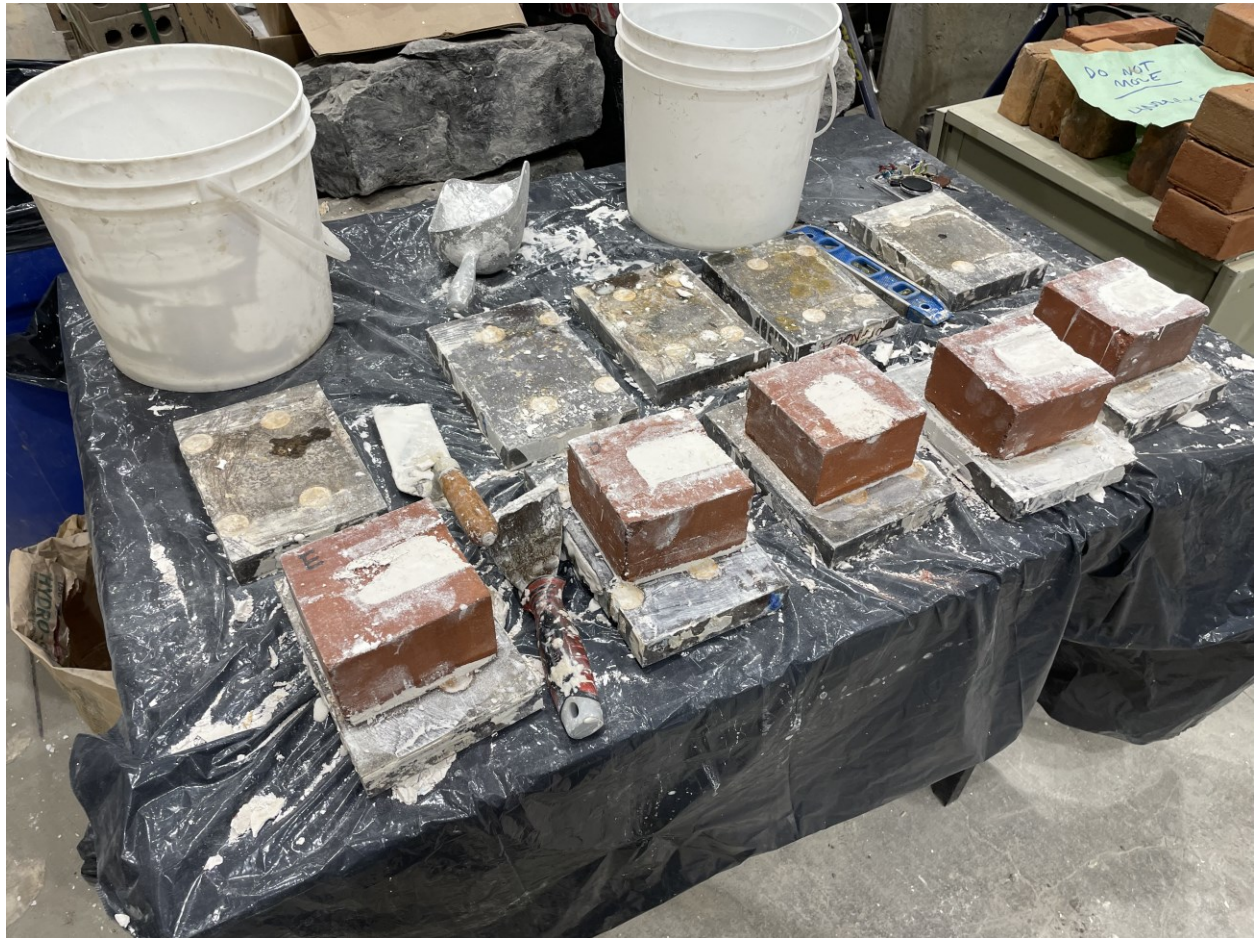
Figure 2.10. Filling the frogs of the MILTON bricks with gypsum cement during the capping process
