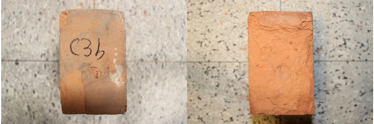
Figure 3.7. CRAIG-3 before and after the freeze-thaw test
