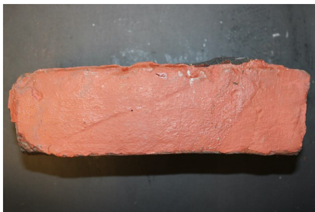
Figure 2.4. Red paint on exposed face of BERRI-NS
