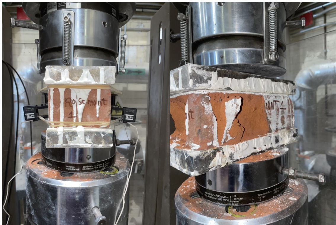
Figure 2.13. Before and after the compression test
