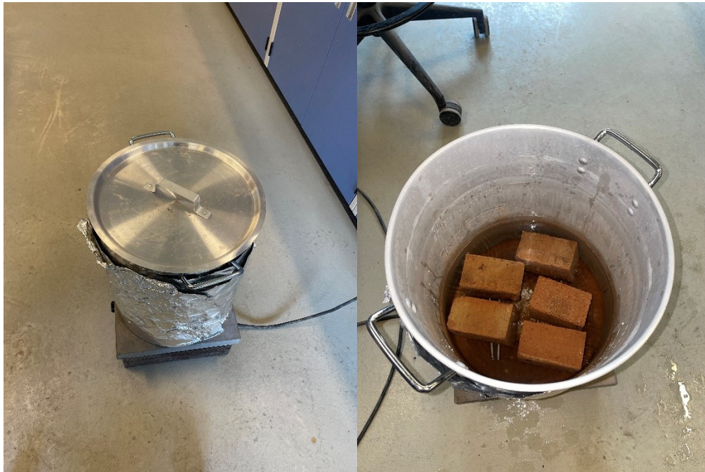
Figure 2.7. 5-h boiling absorption test
