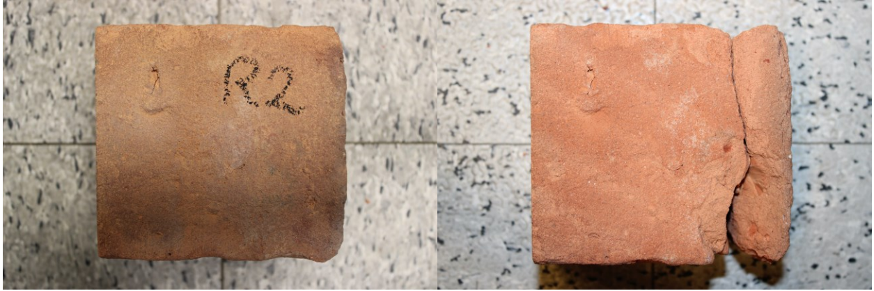
Figure 3.6. ROSEMONT-2 before and after the freeze-thaw test
