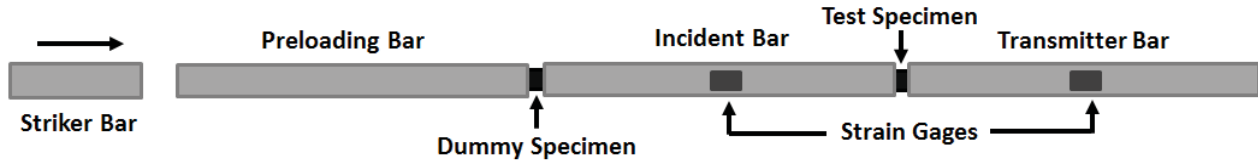
Figure 2.18. Schematic of the three-bar pulse shaping technique 59
