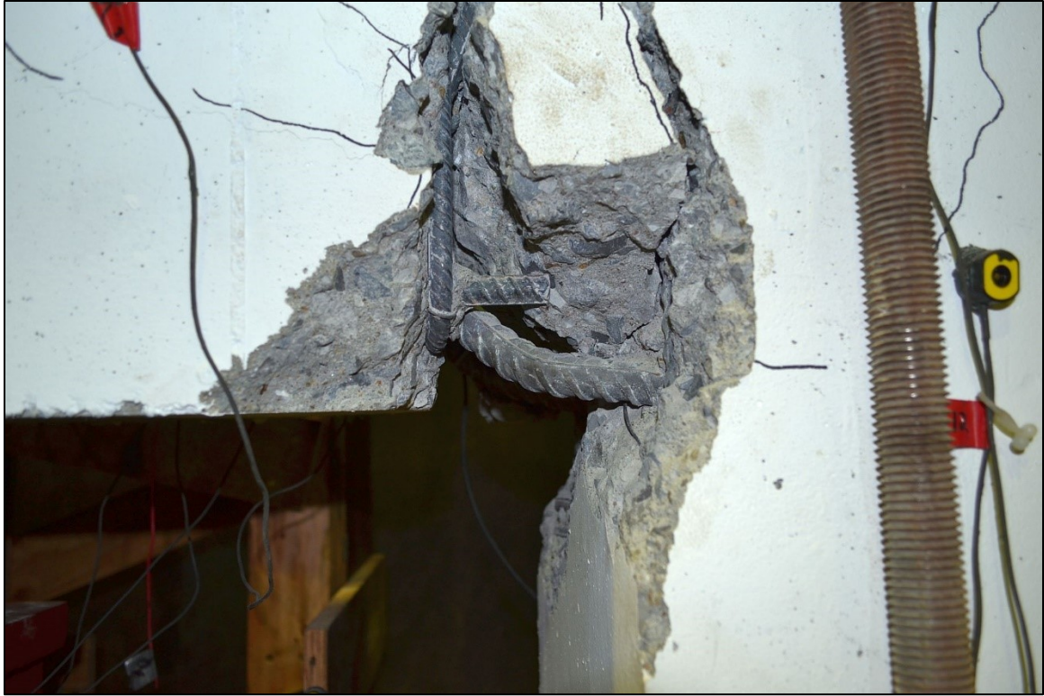
Figure 4.11 – Buckled bar at bottom right coupling beam–coupled wall interface
