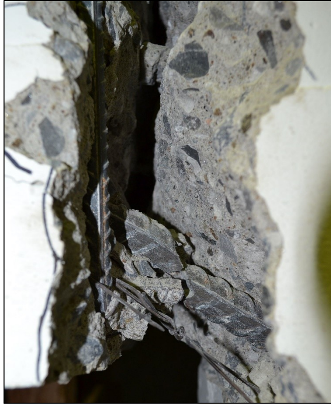
Figure 4.17 – Ruptured bar at bottom right of specimen MD-8d b
