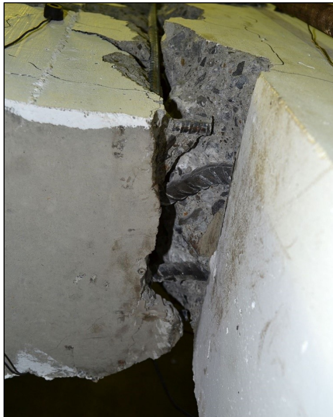
Figure 4.4 – Severe diagonal bar buckling of specimen CC-16d b
