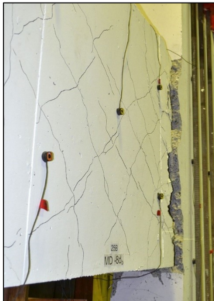
Figure 4.16 – Severe twisting observed at the coupling beam
