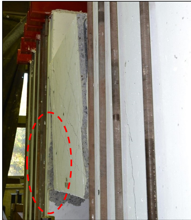
Figure 4.10 – Severe twisting observed at the coupling beam
