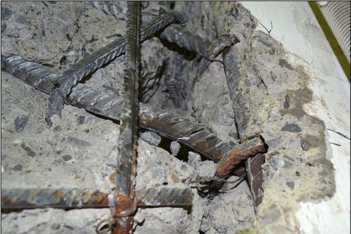
Figure 4.22 – Ruptured bar at bottom right of specimen D-6d b
