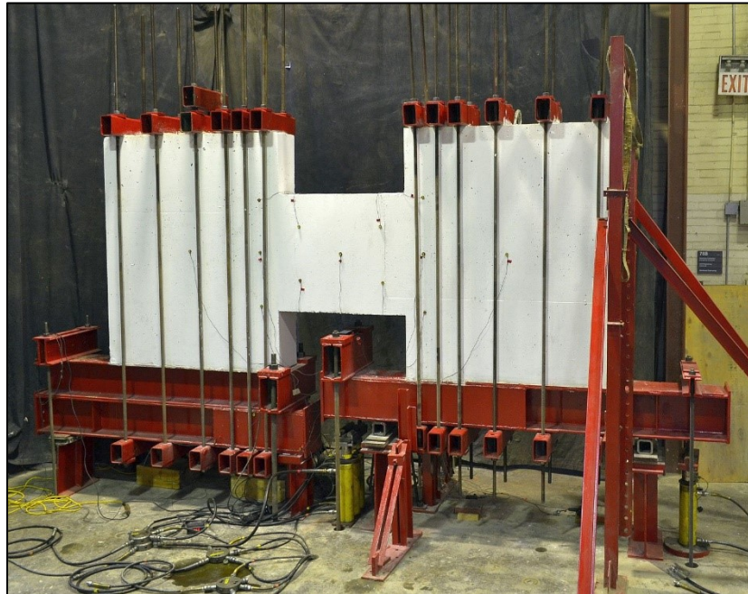
Figure 3.8 – Photograph of McGill University Coupled Wall Testing Apparatus for specimens CC-16d b , MD-10d b and MD-8d b
