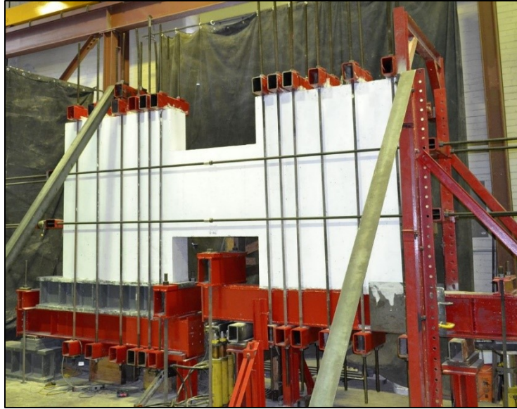
Figure 3.10 – Photograph of McGill University Coupled Wall Testing Apparatus for specimen D-6d b
