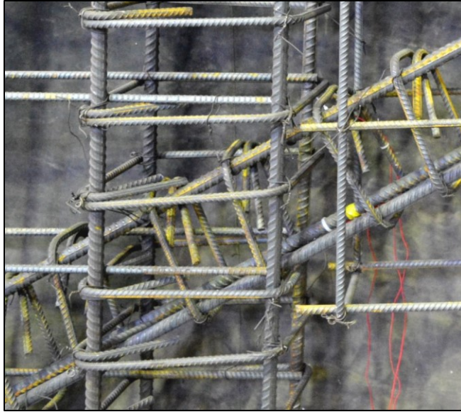
Figure 5.3 –Intertwined concentrated and diagonal reinforcing steel of specimen D-6d b
