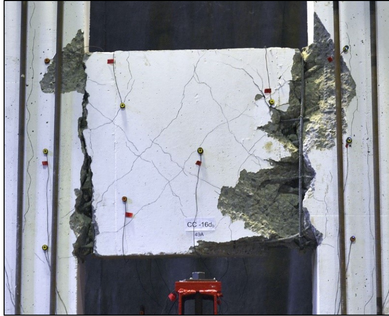
Figure 4.3 – Final load cycle of specimen CC-16d b – 49A
