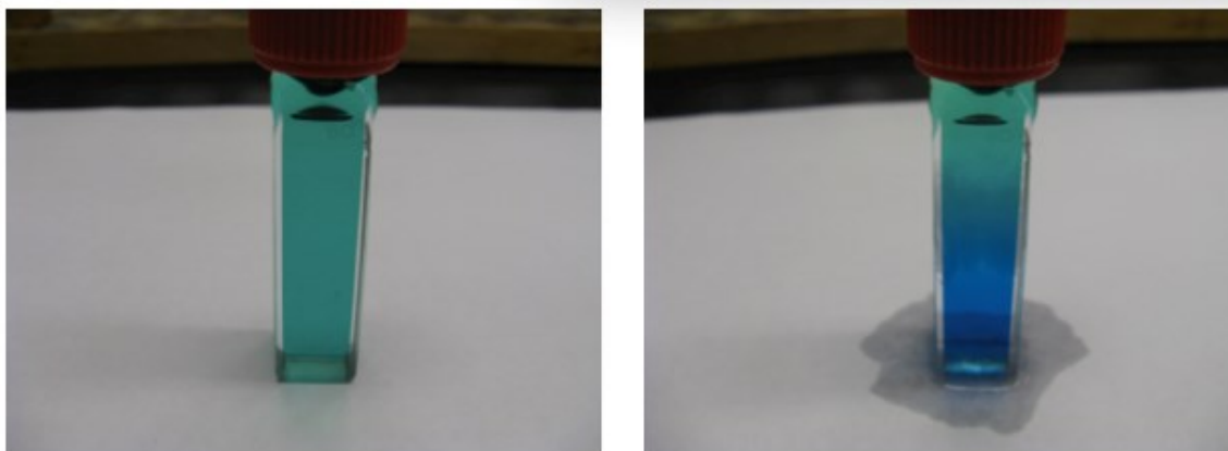
Fig 3.16: A toluene \text{N}_2\text{O}_3 solution at 25^\circ\text{C} (left), then dipped into a -78^\circ\text{C} bath (right).
