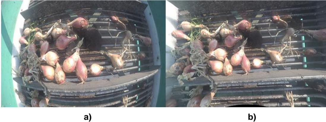
**Figure 3.6.** The distorted image (a) from the Nikon KeyMission 170 camera and the same image that has been undistorted (b). The undistorted image was created using the remapping function of OpenCV.
