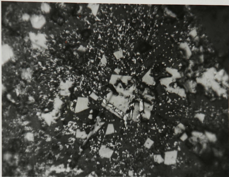
Plate XV. Jaspersy Iron Formation. Chert granule containing hematite (white) and magnetite (light grey). The largest magnetite crystal shows oxidation along octahedral planes. x 280.
