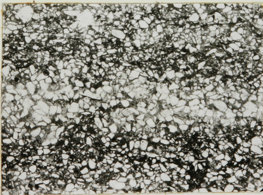
Plate IV. Argillite (lower facies). Same composition as above (with little mica). Bedding prominent because of variation in grain size and composition. Plain light, x 30.
