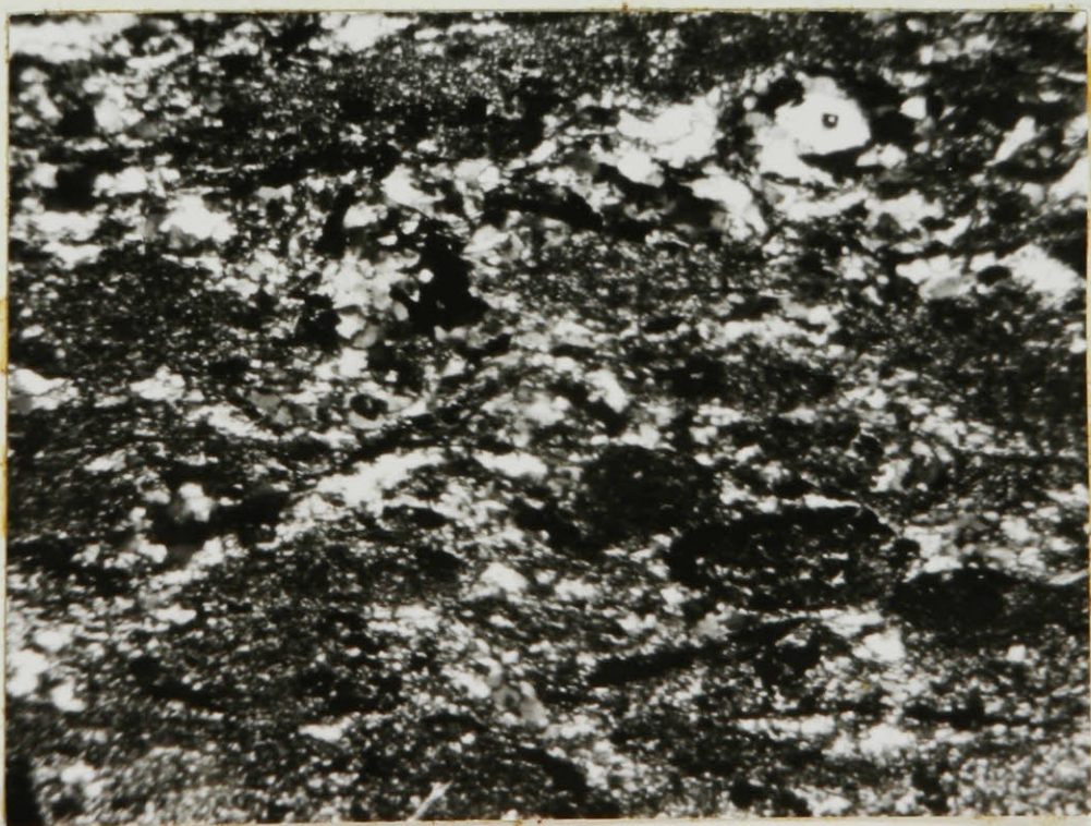
Plate VI. Jaspery Iron Formation. Same type of granules as above as seen between crossed nicols. The chert of the groundmass is coarser grained than the chert of the granules. x 70.
