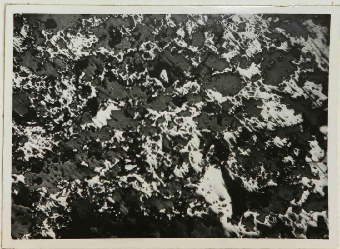
Plate X. Thin-banded Iron Formation. Replacement of chert by hematite. (Same as above). x 280.
