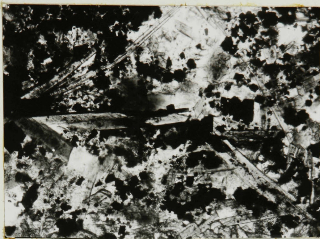
Plate VII. Magnetite Silicate Iron Formation. Intergrowth of the amphibole; riebeckite, (lath-shaped crystals) in a groundmass of chert (white) and fine iron silicate either minnesotaite or stilpnomelane (grey). Also euhedral magnetite (black). Plain light, x 150.
