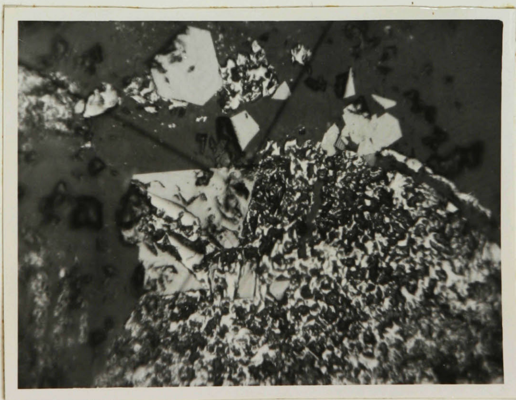
Plate XIV. Jaspery Iron Formation. Part of a granule showing euhedral magne- tite having grown partly in the chert groundmass and in the granule. Some oxidation of the magnetite (light grey) to hematite (white). x 280.
