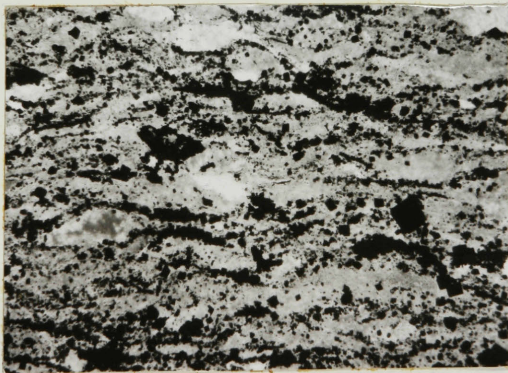
Plate VIII. Magnetite Silicate Iron Formation. Faint granule texture. Fine iron silicate needles either minnesotaite or stilpnomelane (grey) and chert (white). Euhedral magnetite (black) distributed irregularly along bedding planes. Plain light, x 150.
