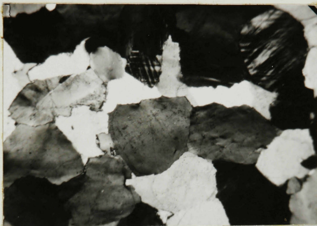
Plate I. Lower Quartzite. Quartz grains cemented together by secondary silica having crystallized in optical continuity. A thin film of secondary iron oxide between interstices (at the left especially). Two feldspar fragments with vague twinning. Crossed nicols, x 70.
