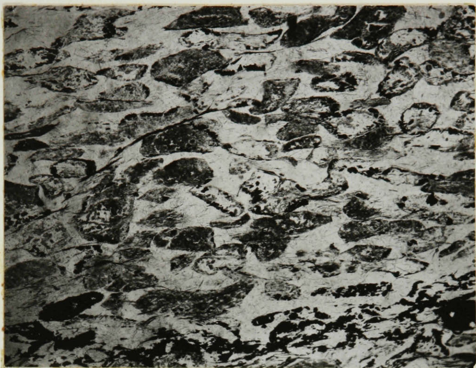
Plate V. Jaspery Iron Formation. Granules composed of chert (light grey) with variable quantity of fine hematite (dark grey). Coarser hematite associated with magnetite appear as black. Note the very fine needles of iron silicates partly altered to goethite and hematite and distributed throughout both granules and groundmass. Plain light, x 40.
