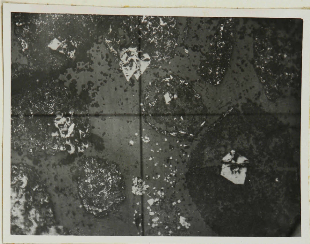
Plate XIII. Jaspery Iron Formation. Chert granules containing irregularly distributed hematite (when fine grained; white). The groundmass is chert (dark grey). Euhedral magnetite present in both granules and groundmass. x 65.
