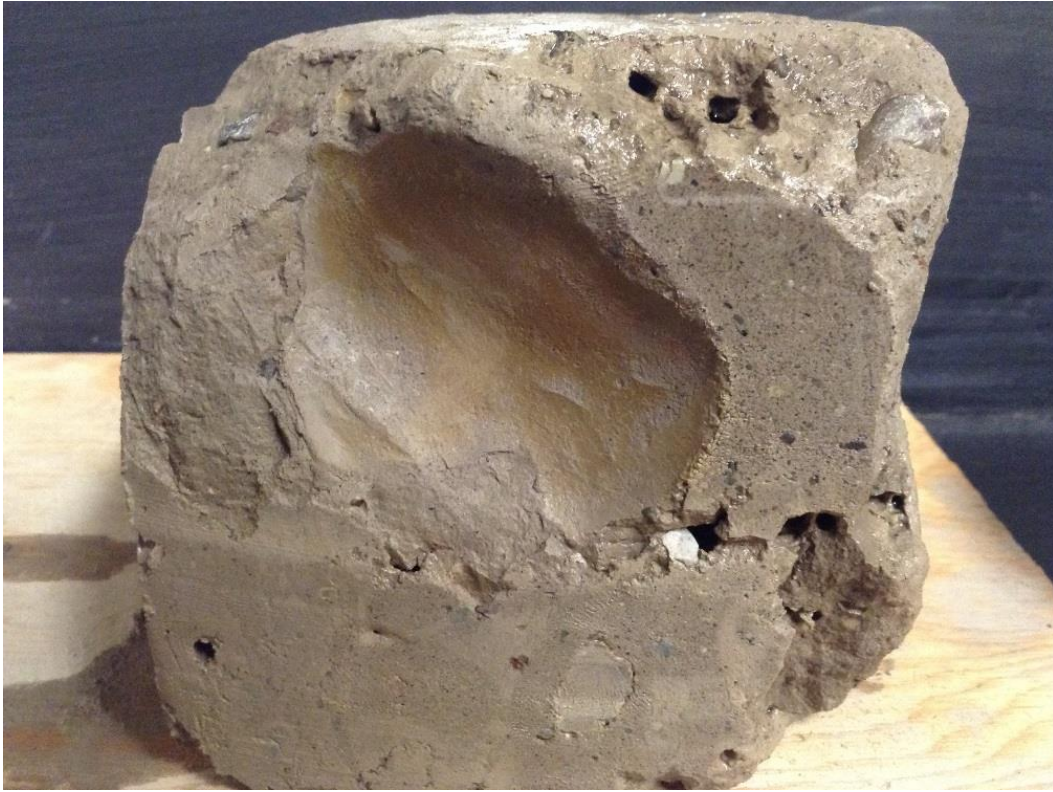
Figure 40: Sample 6 - erosion showing worm holes
