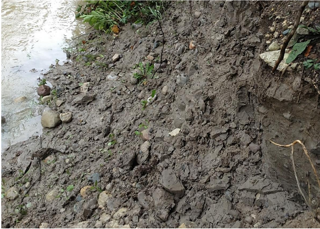
Figure 12: Chunks of till eroded at Medway Creek bank
