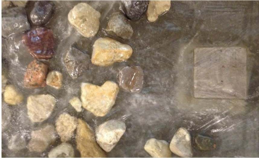
Figure 35: Sample 6 gravel placement with flow < 4.5 L/s
