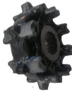
Figure 3 - Drive sprocket with both horizontal and vertical teeth types (removed from drive shaft).
