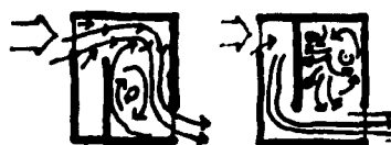
Fig. 35 Effect of internal partition on airflow.
