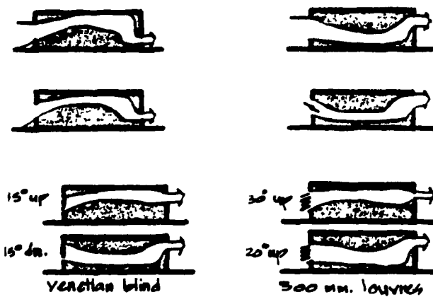
Fig. 33 Effect of canopies, sashes, and louvers on airflow.
