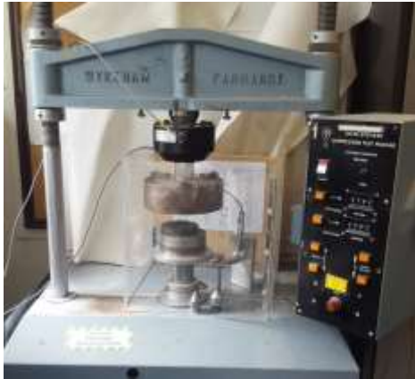
Figure 39. Wykeham Farrance 100 kN mechanical gearbox press machine at the McGill Geomechanics Laboratory.
