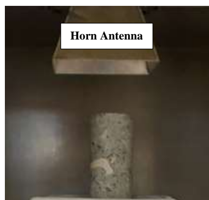
Figure 36. Single-mode microwave cavity in the McGill Geomechanics Laboratory.
