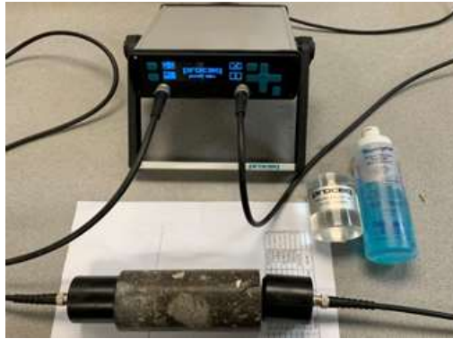
Figure 43. PUNDIT device attached to a rock sample for pulse sound velocity measurement at the McGill Geomechanics Laboratory.
