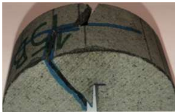
Figure 47. Unacceptable crack propagation within the sample.
