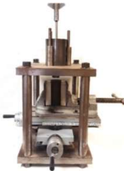
Figure 40. CERCHAR Abrasivity Index apparatus.
