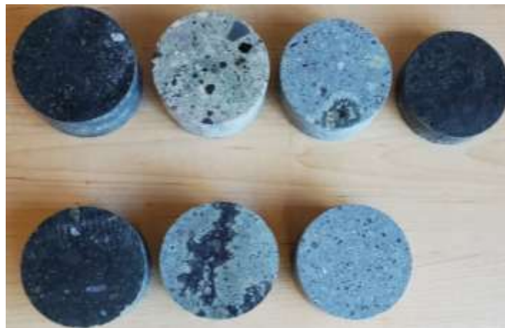
Figure 28. Kimberlite rocks were prepared for dielectric property measurement.
