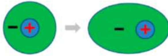
Figure 5. Schematic diagram of electronic polarization(Von Hippel, 1954).
