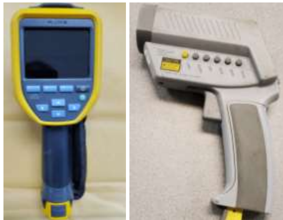
Figure 37. Fluke TiS65 infrared thermal imaging camera (left) and Raytec Raynger MX4+ high-performance infrared gun (right) is located at McGill Geomechanics Laboratory.
