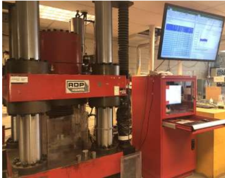
Figure 38. Servo-controlled MTS 250 MN compression machine at the McGill Geomechanics Laboratory.
