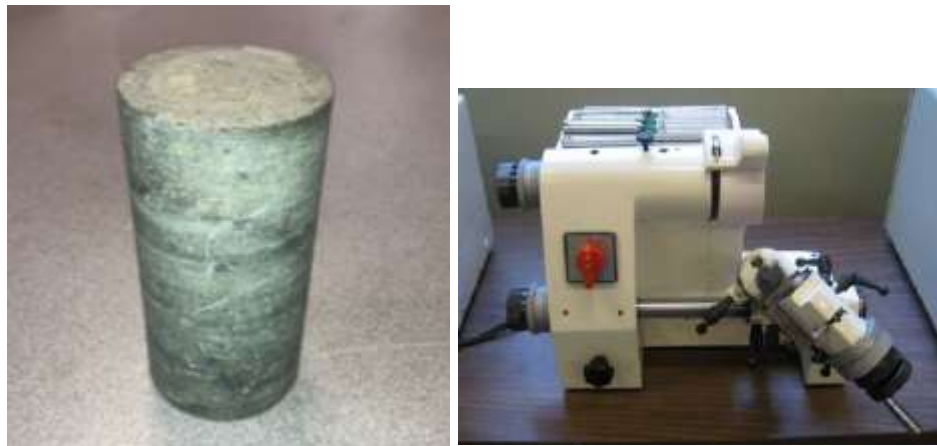
Figure 41. Rock cylindrical sample (left) and Cutter grinder machine(right)
