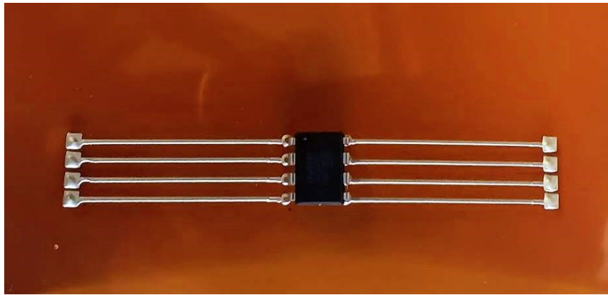
Fig. 4.6 Photo of the prototype on Kapton polyimide.
