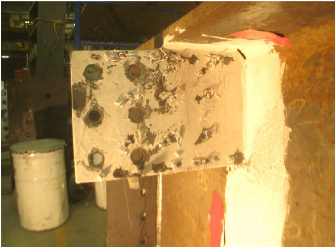
Figure D-127: Shear Tab, End of Test, Configuration 10
