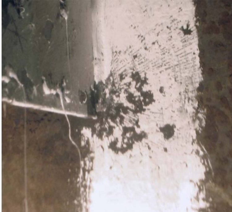
Figure D-118: Yielding of Girder Web at Shear Tab Edge, Configuration 9
