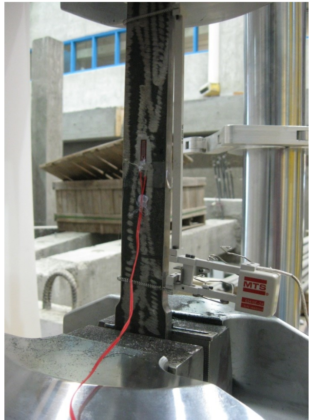
b) Extensometer and Strain Gauge Details
