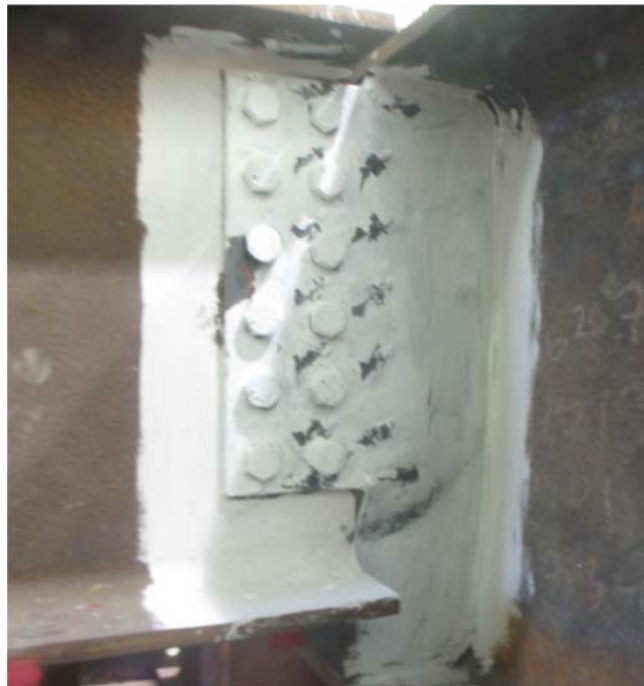
Figure D-144: Deformed Shear Tab, End of Test, Configuration 11
