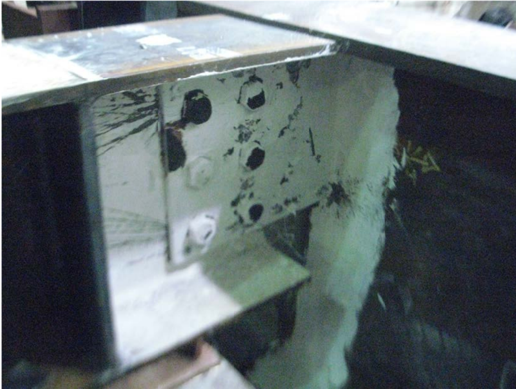
Figure D-80: Shear Tab, End of Test, Configuration 7
