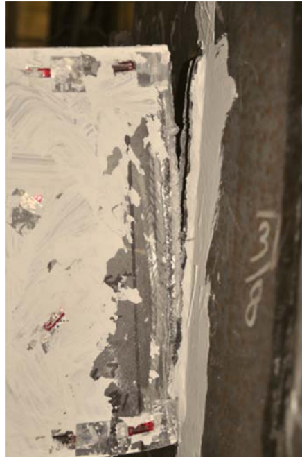
Figure D-9: Weld Tear at End of Test, Configuration 1
