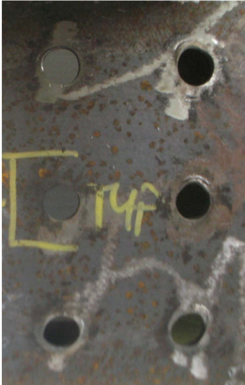
Figure D-92: Beam Bolt Hole Bearing Deformation, Configuration7
