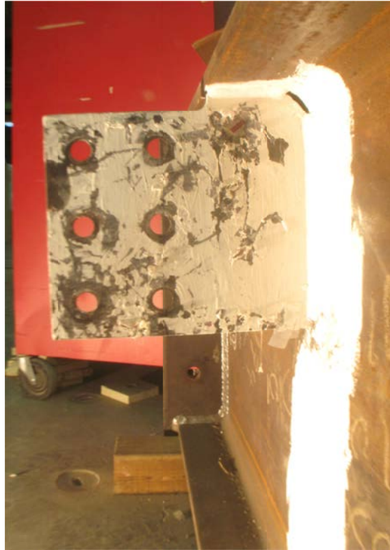
Figure D-65: Unyielded Shear Tab, End of Test, Configuration 6
