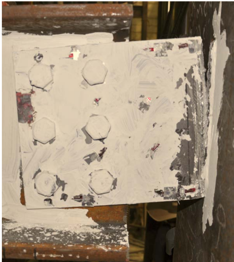
Figure D-4: Yielded Shear Tab, Configuration 1
