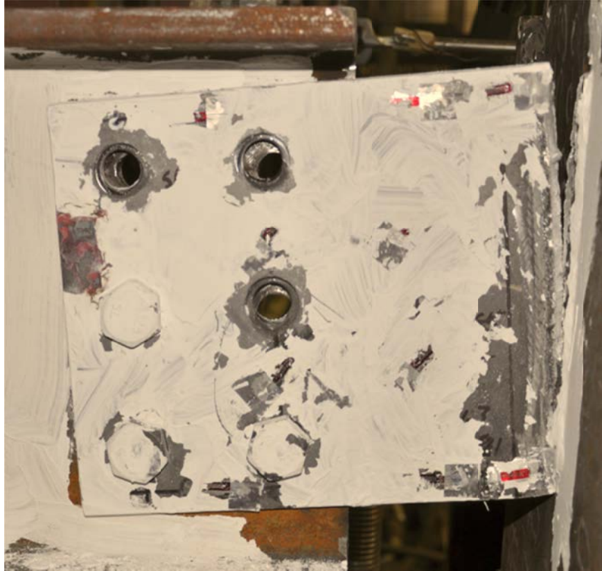
Figure D-10: Shear Tab with Sheared Bolts Removed, Configuration 1
