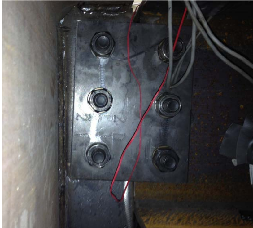
Figure D-105: Bearing Deformation in Girder Stiffener, End of Test, Configuration 8
