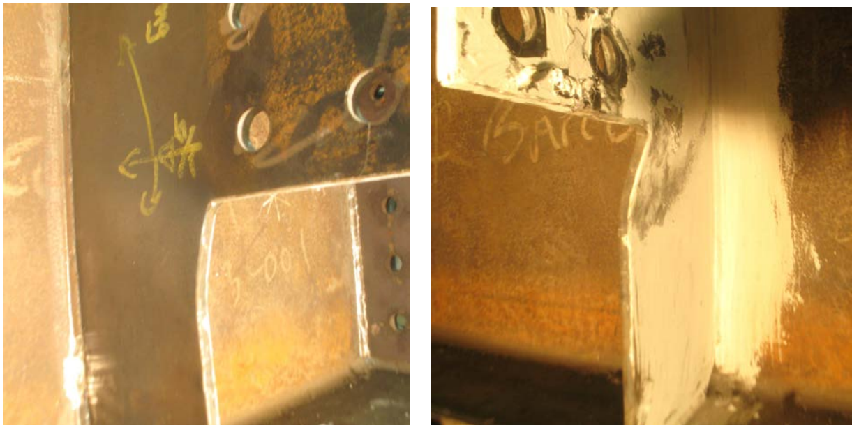
Figure D-142: Buckled Shear Tab Neck, Various Angles, Configuration 11
