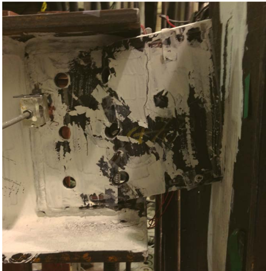
Figure D-28: Yielded Shear Tab, Configuration 3
