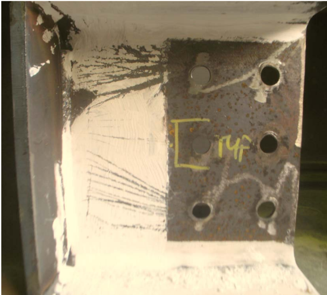
Figure D-89: Tension Field on Beam Web, End of Test, Configuration 7
