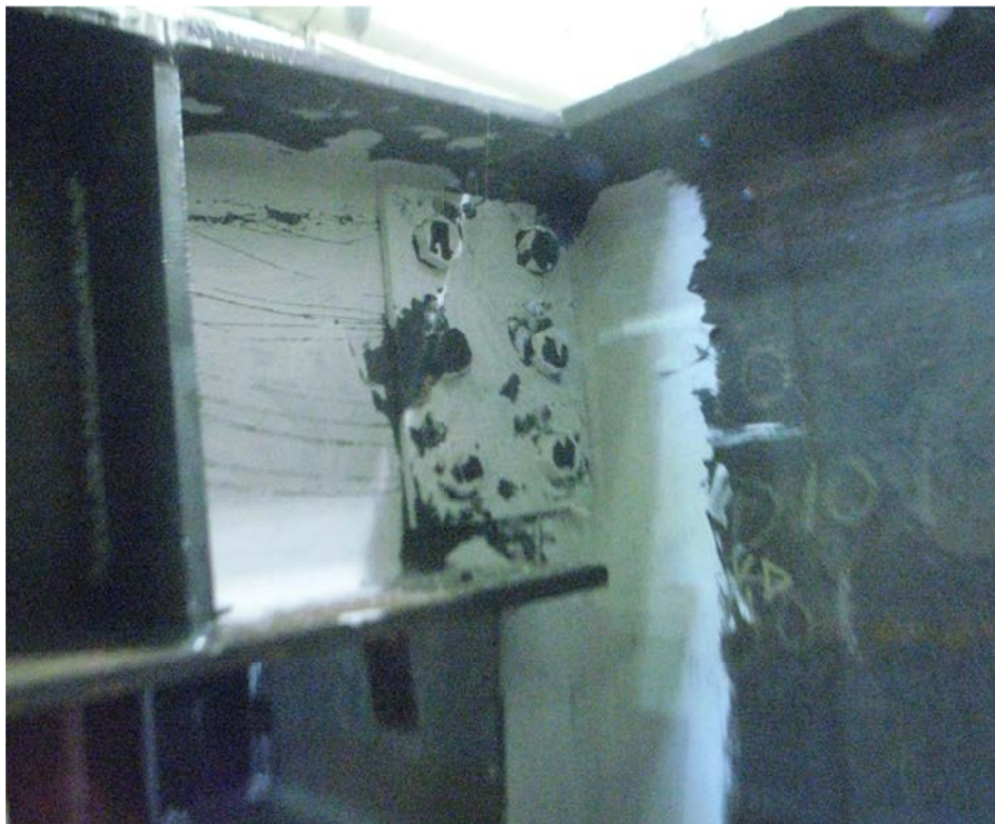
Figure D-96: Deformed Condition, End of Test, Configuration 8
