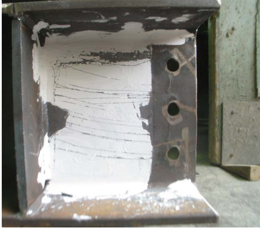
Figure D-107: Tension Field on Beam Web, End of Test, Configuration 8
