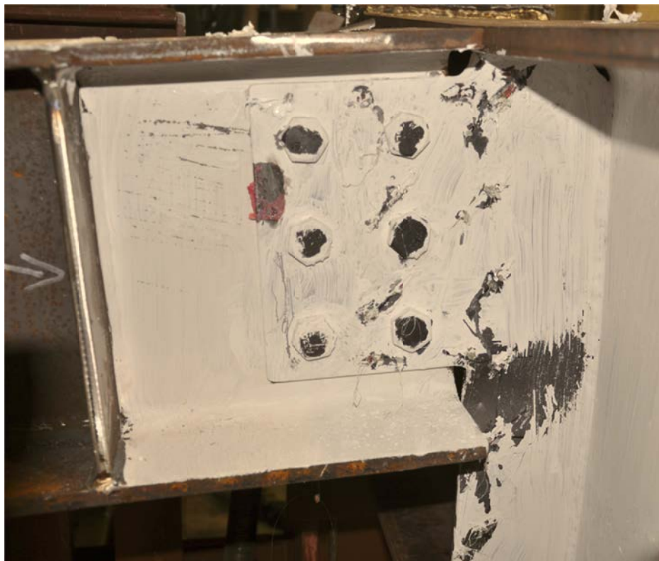
Figure D-56: Deformed Shear Tab, End of Test, Configuration 5
