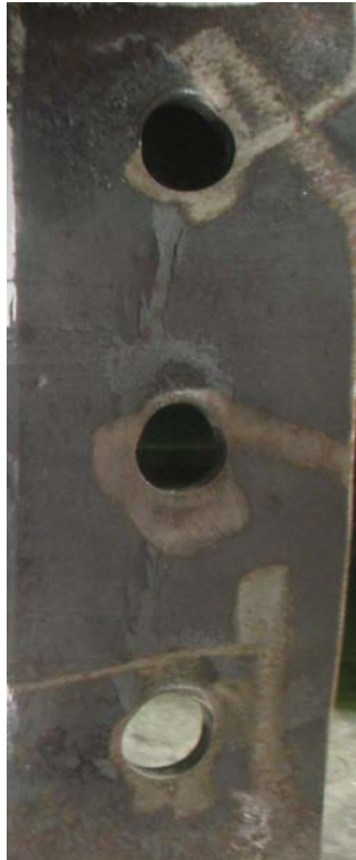
Figure 106: Deformed Bolt Holes, Beam and Stiffener, Configuration 8
