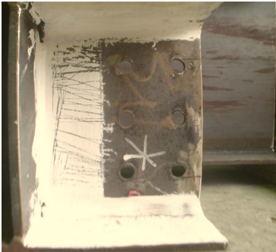
Figure D-136: Tension Field on Beam Web, End of Test, Configuration 10
