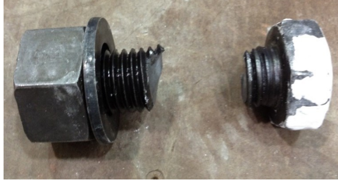
Figure 4.9: Sheared Bolt, Configuration 1
