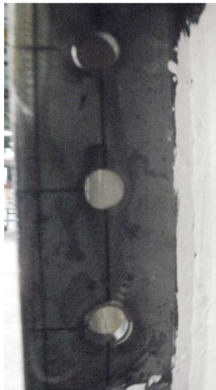
Figure 106: Deformed Bolt Holes, Beam and Stiffener, Configuration 8
