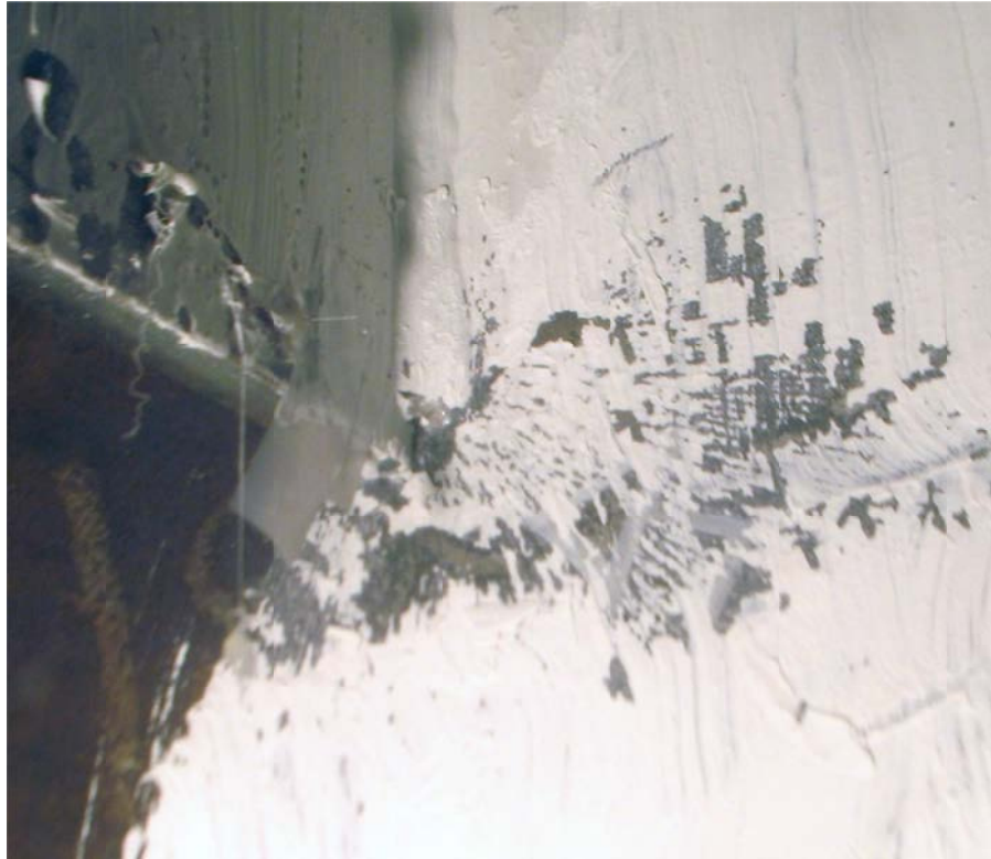
Figure D-70: Yielding of Girder Web at Shear Tab Edge, Configuration 6
