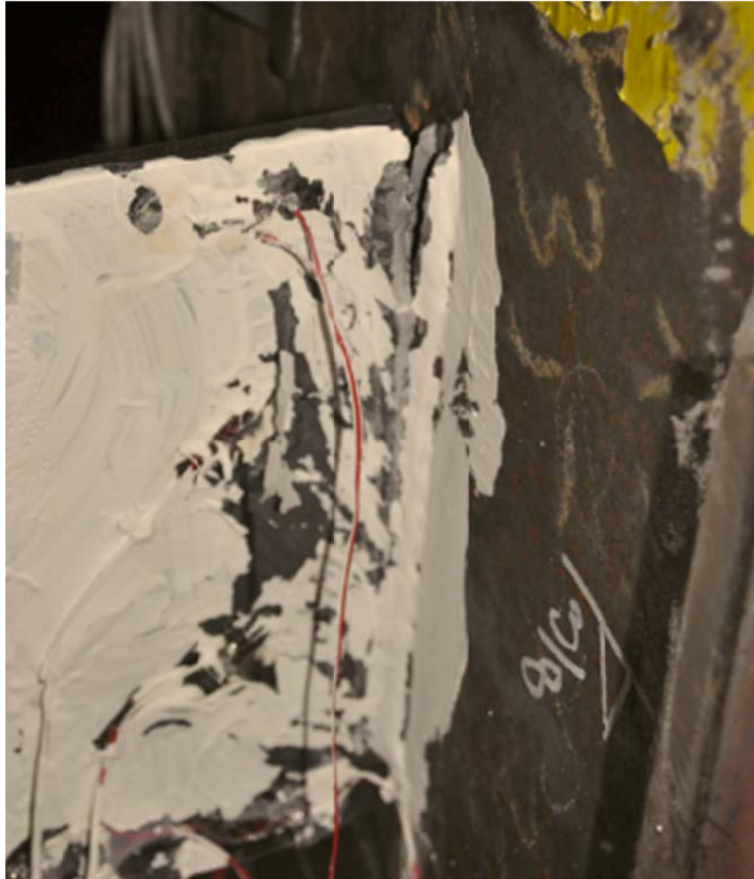
Figure D-23: Weld Tearing, End of Test, Configuration 2
