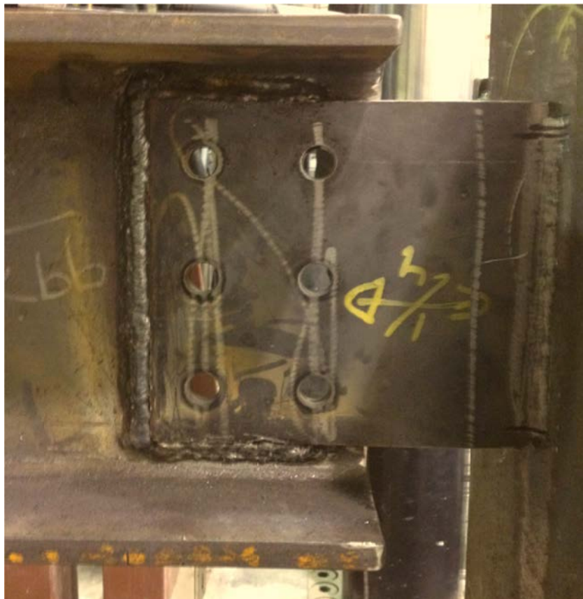
Figure D-26: Partial "C" Weld, Before Test, Configuration 3
