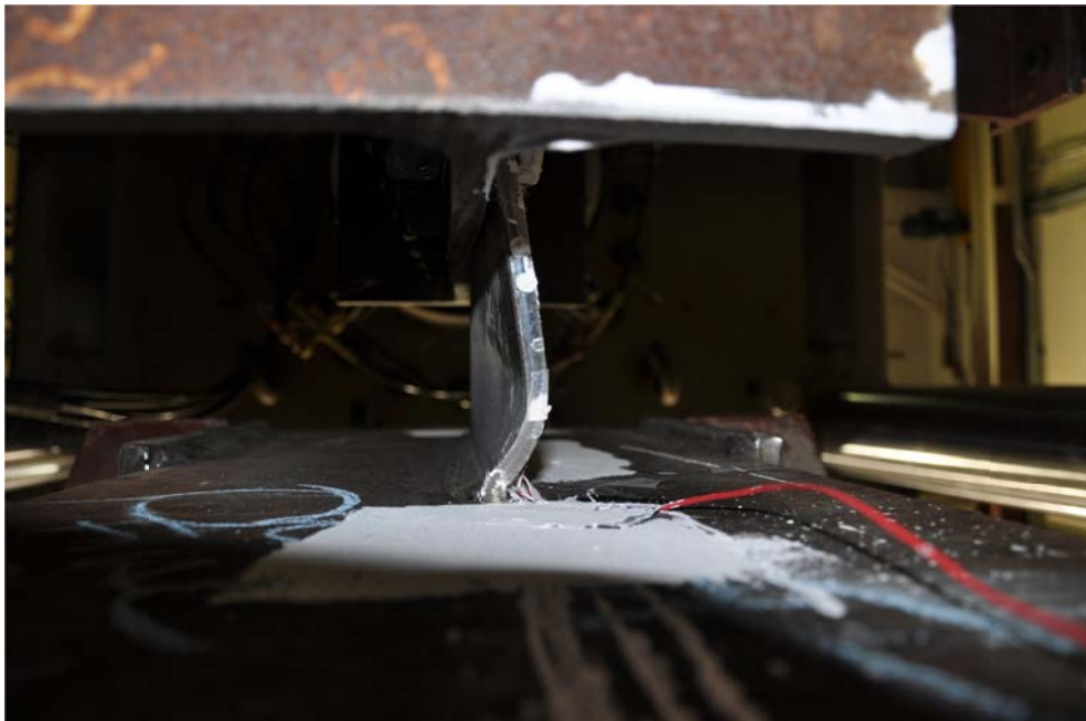
Figure D-47: Buckled Shear Tab, End of Test (photo from below beam), Configuration 4
