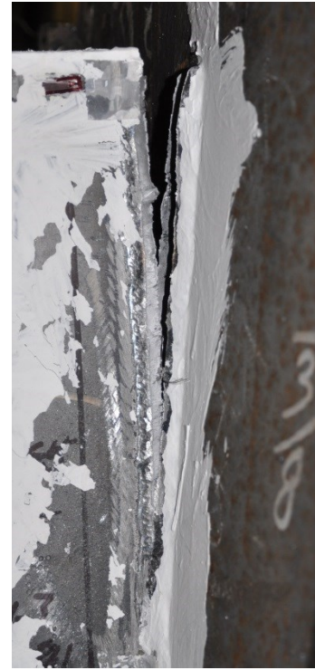
b) Weld Fracture Detail
