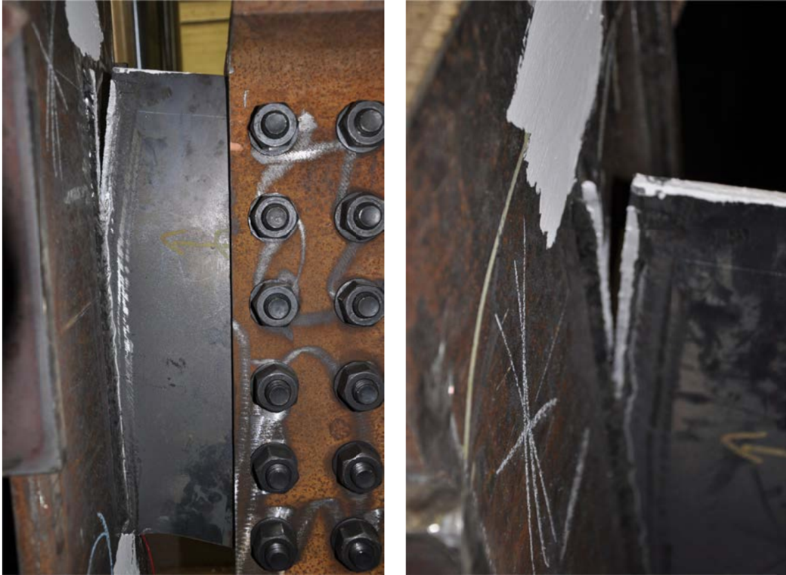
Figure D-48: Weld Tearing, End of Test, Configuration 4
