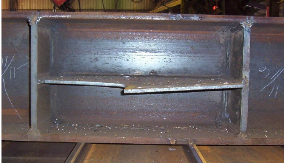
Figure 2.19: Buckled Shear Tab, Test 1, Goodrich (2005)
