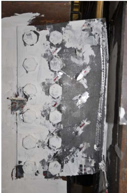
Figure D-40: Yielded Shear Tab, Configuration 4
