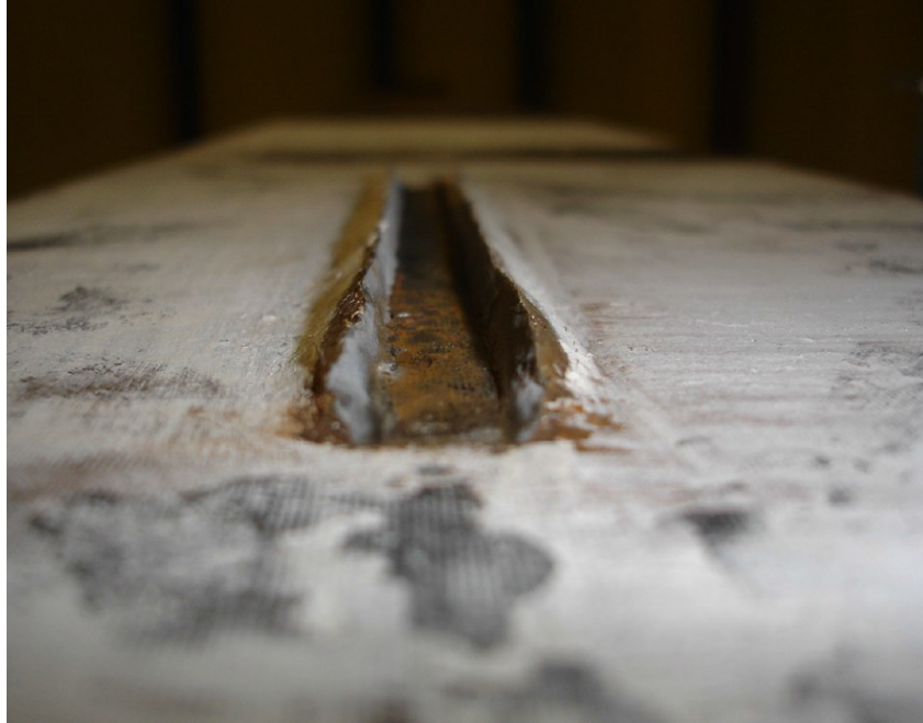
Figure 2.20: Weld Rupture, Test 5b, Baldwin Metzger (2006)
