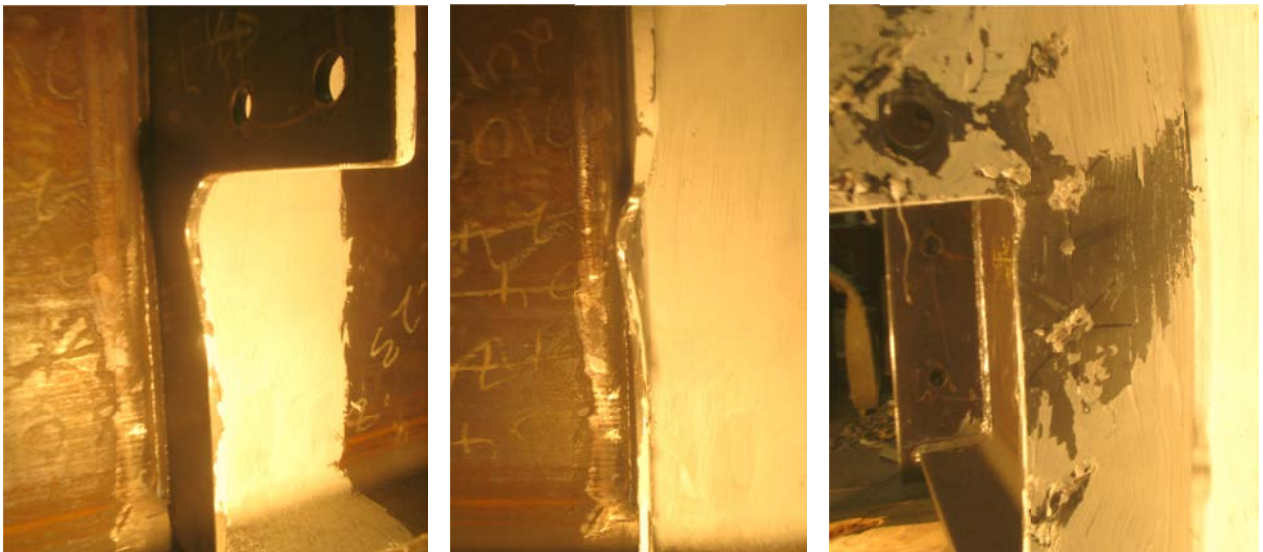
Figure D-54: Buckled Shear Tab Neck, Various Angles, Configuration 5
