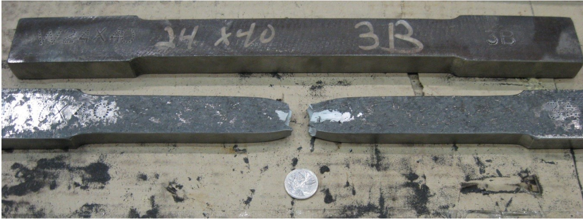
Figure 4.3: Coupon Specimens Before (W24x94 Flange) and After (W27x84 Flange) Uniaxial Tensile Test
