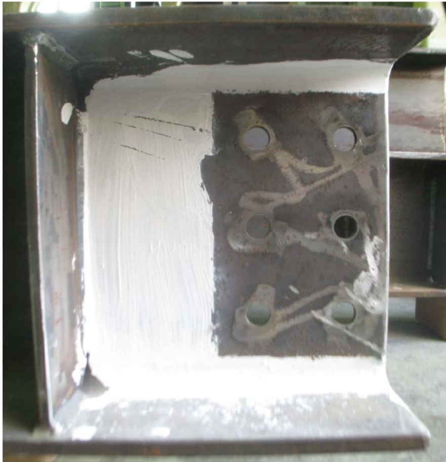
Figure D-74: Tension Field on Beam Web, End of Test, Configuration 6
