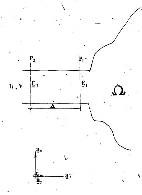
FIG 4.4 THE PORT PLANE AT PORT i
