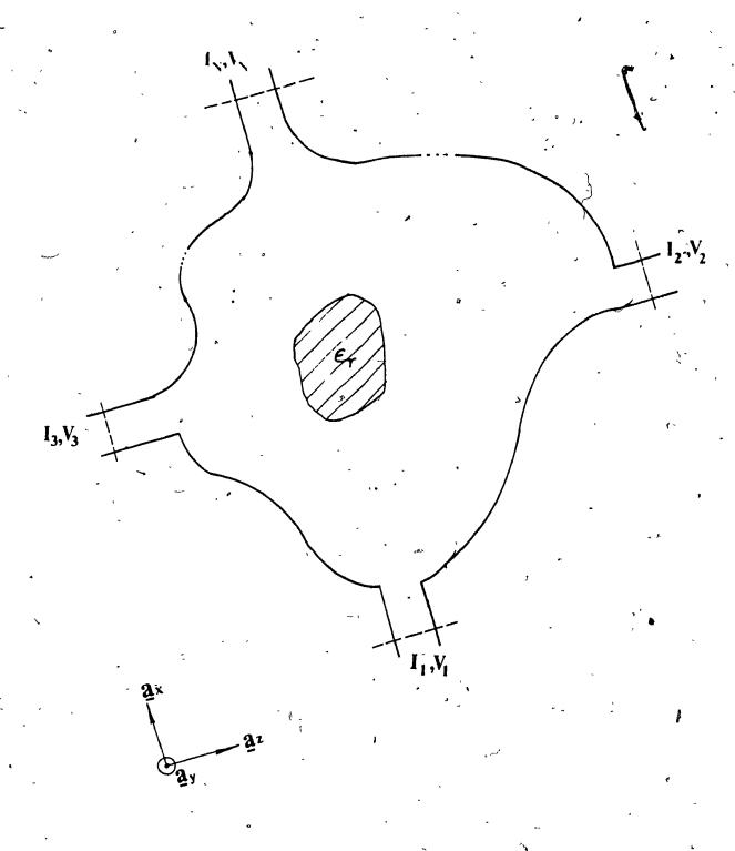
⟨FIG 3.2 A WAVEGUIDE JUNCTION
