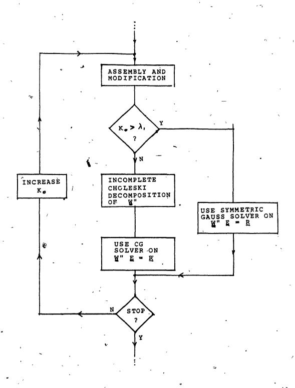
FIG 6.2 A FLOW DIAGRAM THAT EXPLOITS THE POSITIVE DEFINITE PROPERTY OF W.", WHEN POSSIBLE
