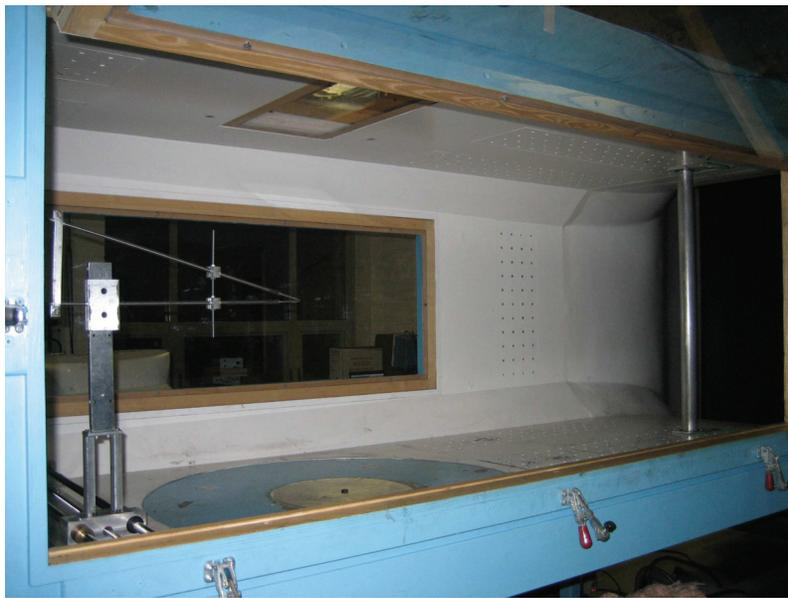
Figure 2.2: Picture of the open-circuit wind tunnel test section with the current experimental apparatus installed. The hot- and cold-wire probes are mounted on a stepper-motor-controlled traversing mechanism, which enables the probes to travel in the transverse (i.e.  $y$ -) direction.
