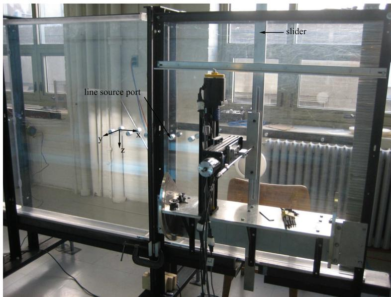
Figure 2.4: Picture of the modified channel test section with a sliding access port for the hot- and cold-wire sensors. The latter were positioned by a two-axis linear traversing mechanism, enabling movement in the  $y$  (transverse) and  $z$  (lateral) directions.
