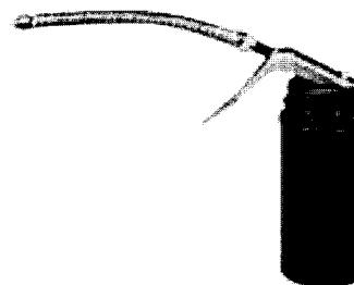
Figure 6.38. A pistol oiler.
