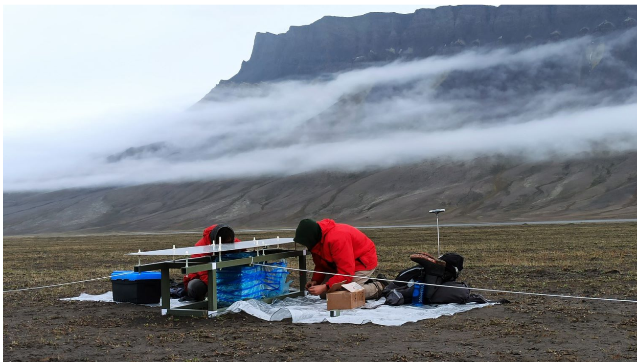
Figure 2.4: MIST installation process at Axel Heiberg island in July 2022. The blue plastic wrap was used to protect the instrument from bad weather conditions.
