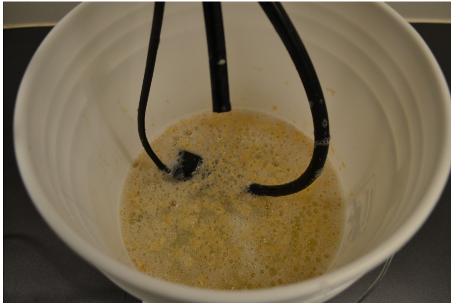
Figure 5: Contaminated nutrient tank at the end of system operation
