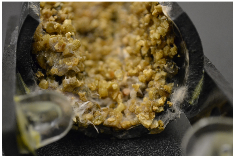
Figure 4: Mycelium growth at the base and sides of the tube encasement
