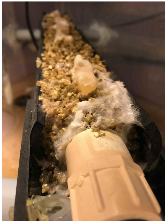
Figure 3: Most significant growth mass of mycelium from the system operation
