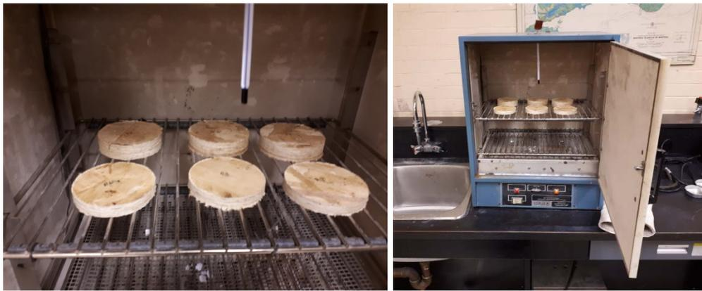
Figure D.55: Oven-dry method for moisture content measurements
