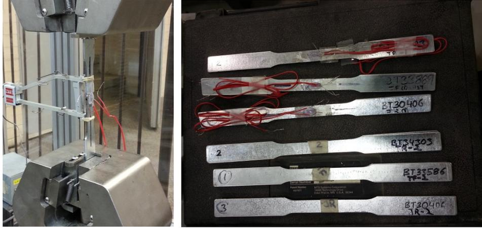
Figure D.54: Tensile coupon tests
