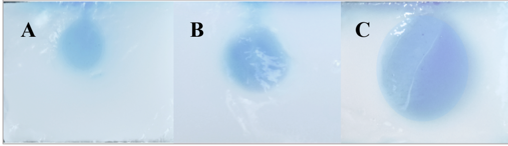
Figure 37: Liquid dispersion profile for fluid delivered at volumes of (A) 0.05 mL, (B) 0.1 mL, and (C) 0.2 mL.
