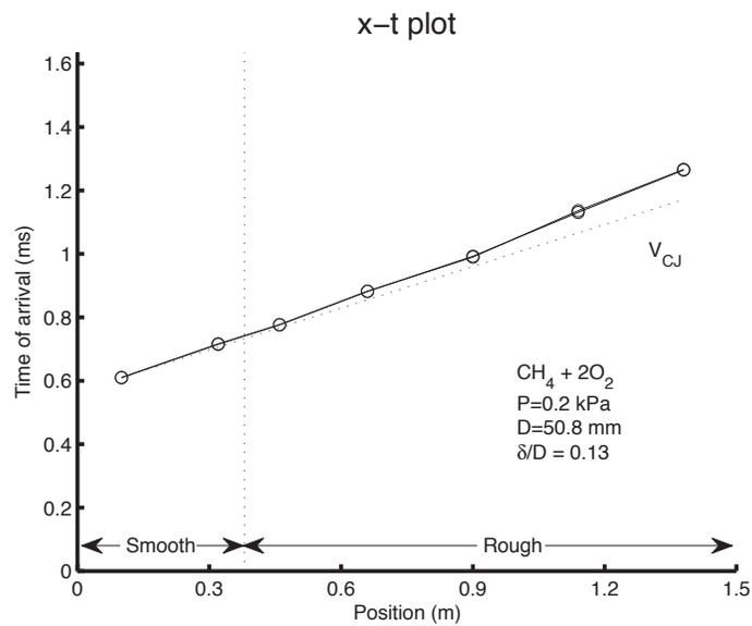
Figure A-7: Detonation Trajectory for  $CH_4 + 2O_2$  in the 50.8 mm tube with  $\delta/D = 0.13$  at a pressure of 12 kPa
