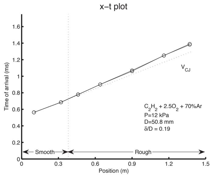
Figure A-6: Detonation Trajectory for  $C_2H_2 + 2.5O_2 + 70\% Ar$  in the 50.8 mm tube with  $\delta/D = 0.19$  at a pressure of 12 kPa
