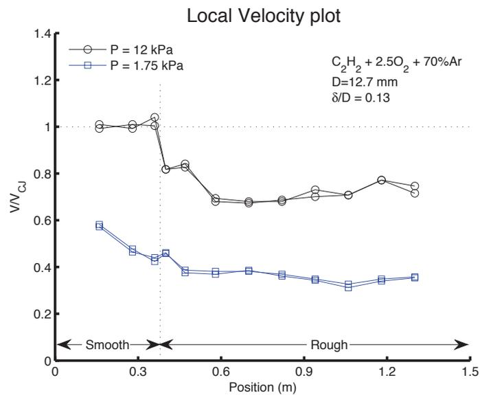
Figure 3–2: Local velocities for  $C_2H_2 + 2.5O_2 + 70\% Ar$  in the 12.7 mm tube with  $\delta/D = 0.13$  with varying pressures showing the progression towards the limit
