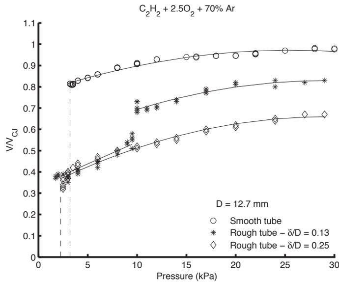
Figure 3-3:  $V/V_{CJ}$  vs. Pressure for  $C_2H_2 + 2.5O_2 + 70\% Ar$  in the 12.7 mm diameter tube
