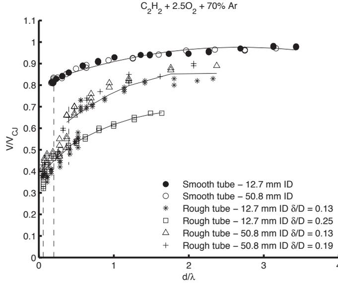
Figure 3-7:  $V/V_{CJ}$  vs.  $d/\lambda$  for  $C_2H_2 + 2.5O_2 + 70\% Ar$
