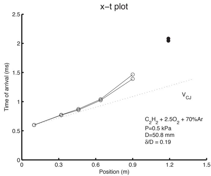
Figure A-14: Detonation Trajectory for  $C_2H_2 + 2.5O_2 + 70\% Ar$  in the 50.8 mm tube with  $\delta/D = 0.19$  at the limit pressure of 0.5 kPa
