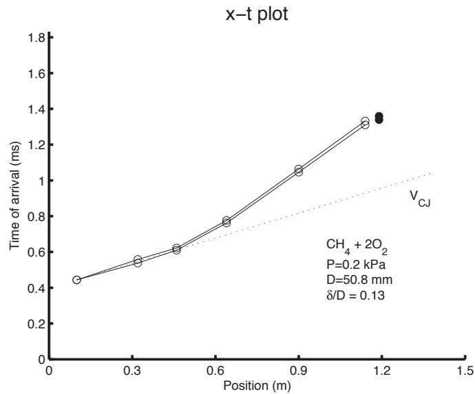
Figure A-15: Detonation Trajectory for  $CH_4 + 2O_2$  in the 50.8 mm tube with  $\delta/D = 0.13$  at the limit pressure of 0.2 kPa
