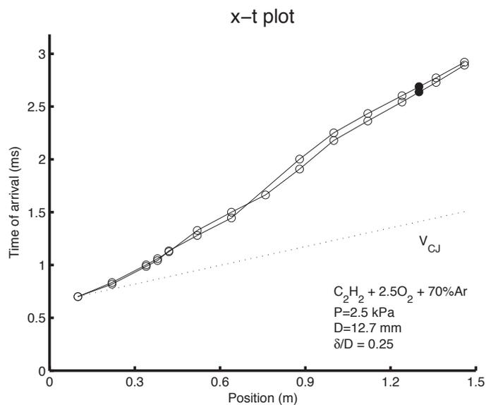
Figure A-10: Detonation Trajectory for  $C_2H_2 + 2.5O_2 + 70\% Ar$  in the 12.7 mm tube with  $\delta/D = 0.25$  at the limit pressure of 2.5 kPa
