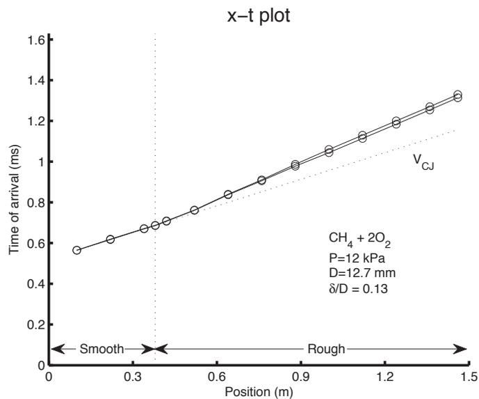
Figure A-3: Detonation Trajectory for  $CH_4 + 2O_2$  in the 12.7 mm tube with  $\delta/D = 0.13$  at a pressure of 12 kPa
