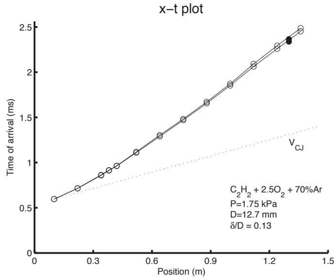
Figure A-9: Detonation Trajectory for  $C_2H_2 + 2.5O_2 + 70\% Ar$  in the 12.7 mm tube with  $\delta/D = 0.13$  at the limit pressure of 1.75 kPa
