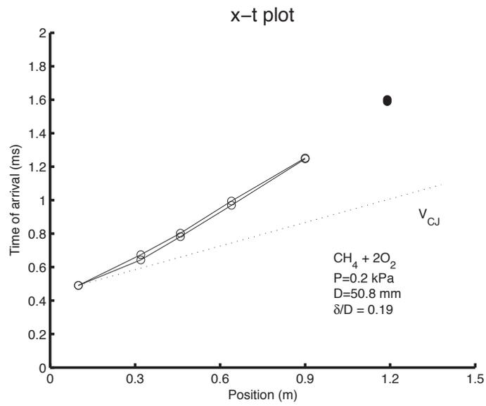
Figure A-16: Detonation Trajectory for  $\text{CH}_4 + 2\text{O}_2$  in the 50.8 mm tube with  $\delta/D = 0.19$  at the limit pressure of 0.2 kPa
