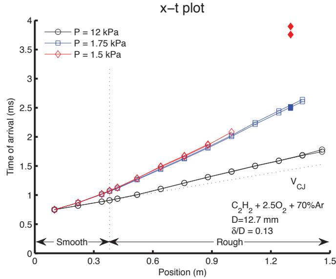
Figure 3–1: Detonation trajectories for  $C_2H_2 + 2.5O_2 + 70\% Ar$  in the 12.7 mm diameter tube with  $\delta/D = 0.13$  with varying pressures showing the progression towards the limit
