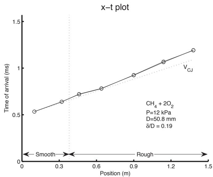
Figure A-8: Detonation Trajectory for  $\text{CH}_4 + 2\text{O}_2$  in the 50.8 mm tube with  $\delta/D = 0.19$  at a pressure of 12 kPa
