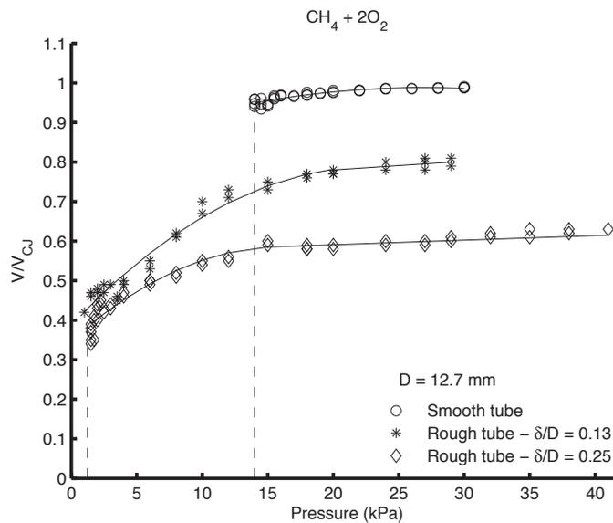
Figure 3–5:  $V/V_{CJ}$  vs. Pressure for  $\text{CH}_4 + 2\text{O}_2$  in the 12.7 mm diameter tube
