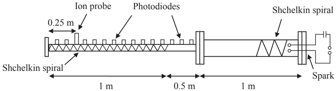
Figure 2–1: Schematic of Experimental Set-Up
