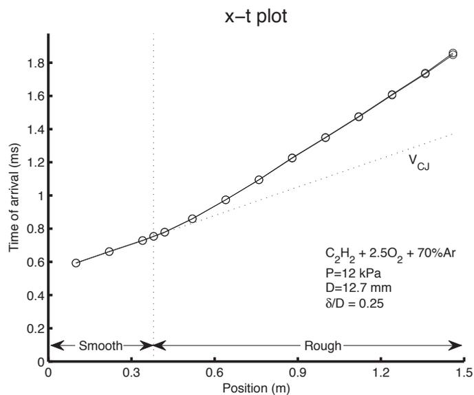
Figure A-2: Detonation Trajectory for  $C_2H_2 + 2.5O_2 + 70\% Ar$  in the 12.7 mm tube with  $\delta/D = 0.25$  at a pressure of 12 kPa
