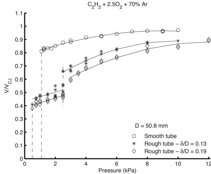
Figure 3-4:  $V/V_{CJ}$  vs. Pressure for  $C_2H_2 + 2.5O_2 + 70\% Ar$  in the 50.8 mm diameter tube
