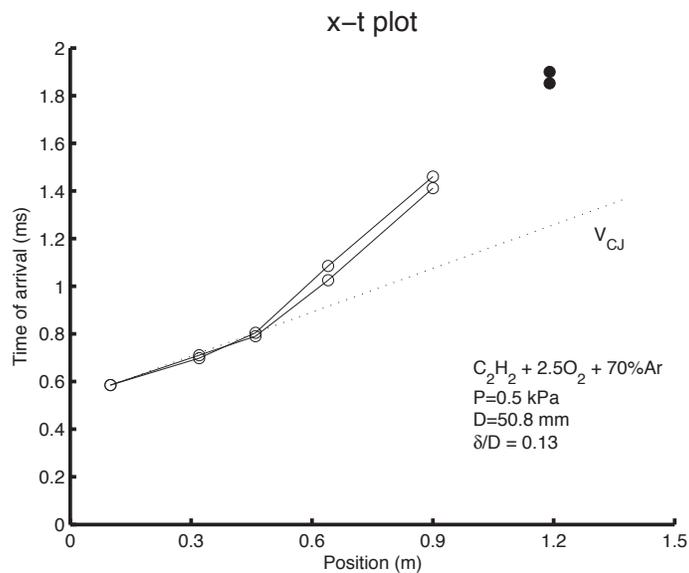
Figure A-13: Detonation Trajectory for  $\text{C}_2\text{H}_2 + 2.5\text{O}_2 + 70\% \text{Ar}$  in the 50.8 mm tube with  $\delta/D = 0.13$  at the limit pressure of 0.5 kPa
