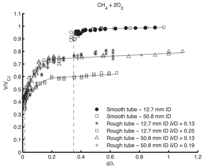
Figure 3–8:  $V/V_{CJ}$  vs.  $d/\lambda$  for  $\text{CH}_4 + 2\text{O}_2$
