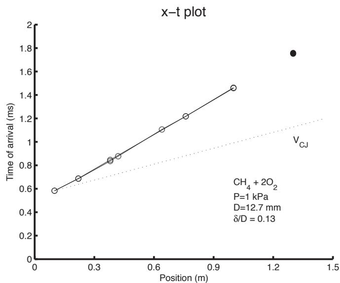
Figure A-11: Detonation Trajectory for  $CH_4 + 2O_2$  in the 12.7 mm tube with  $\delta/D = 0.13$  at the limit pressure of 1 kPa
