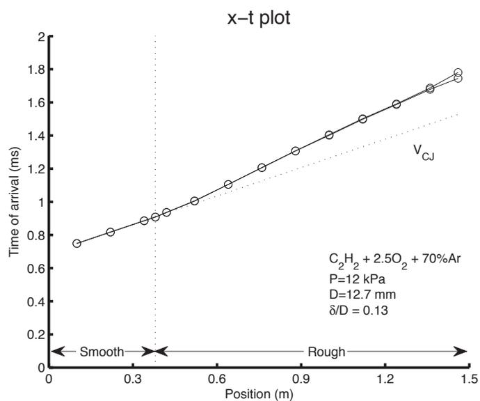
Figure A-1: Detonation Trajectory for  $C_2H_2 + 2.5O_2 + 70\% Ar$  in the 12.7 mm tube with  $\delta/D = 0.13$  at a pressure of 12 kPa
