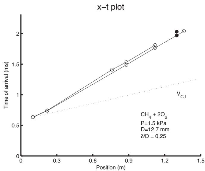
Figure A-12: Detonation Trajectory for  $\text{CH}_4 + 2\text{O}_2$  in the 12.7 mm tube with  $\delta/D = 0.25$  at the limit pressure of 1.5 kPa
