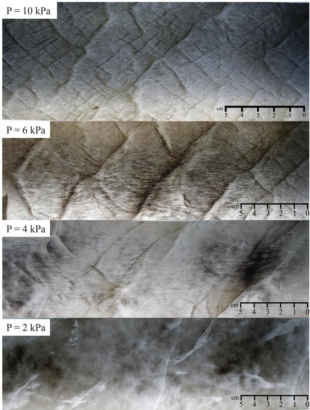
Figure 3–9: Smoked foils for  $\text{C}_2\text{H}_2 + 2.5\text{O}_2 + 70\% \text{ Ar}$  in the 50.8 mm diameter tube with  $\delta/D = 0.13$
