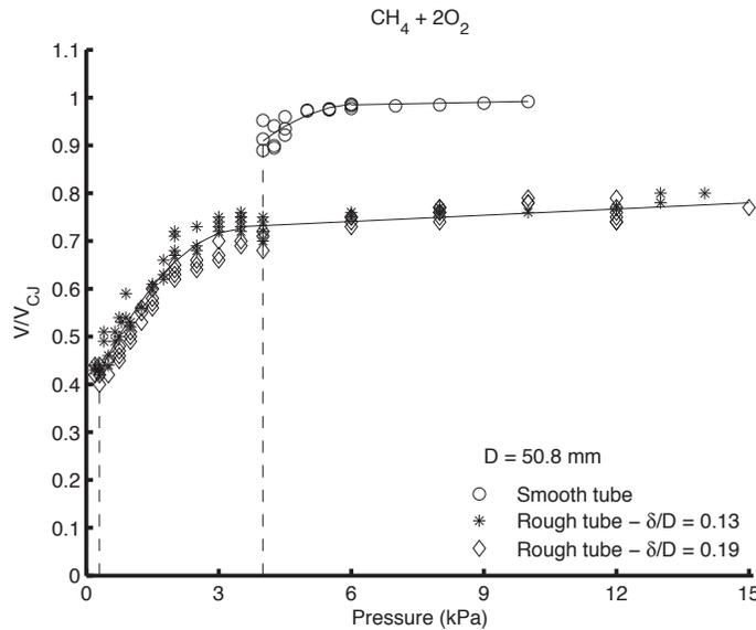
Figure 3-6:  $V/V_{CJ}$  vs. Pressure for  $\text{CH}_4 + 2\text{O}_2$  in the 50.8 mm diameter tube
