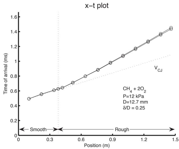
Figure A-4: Detonation Trajectory for  $\text{CH}_4 + 2\text{O}_2$  in the 12.7 mm tube with  $\delta/D = 0.25$  at a pressure of 12 kPa
