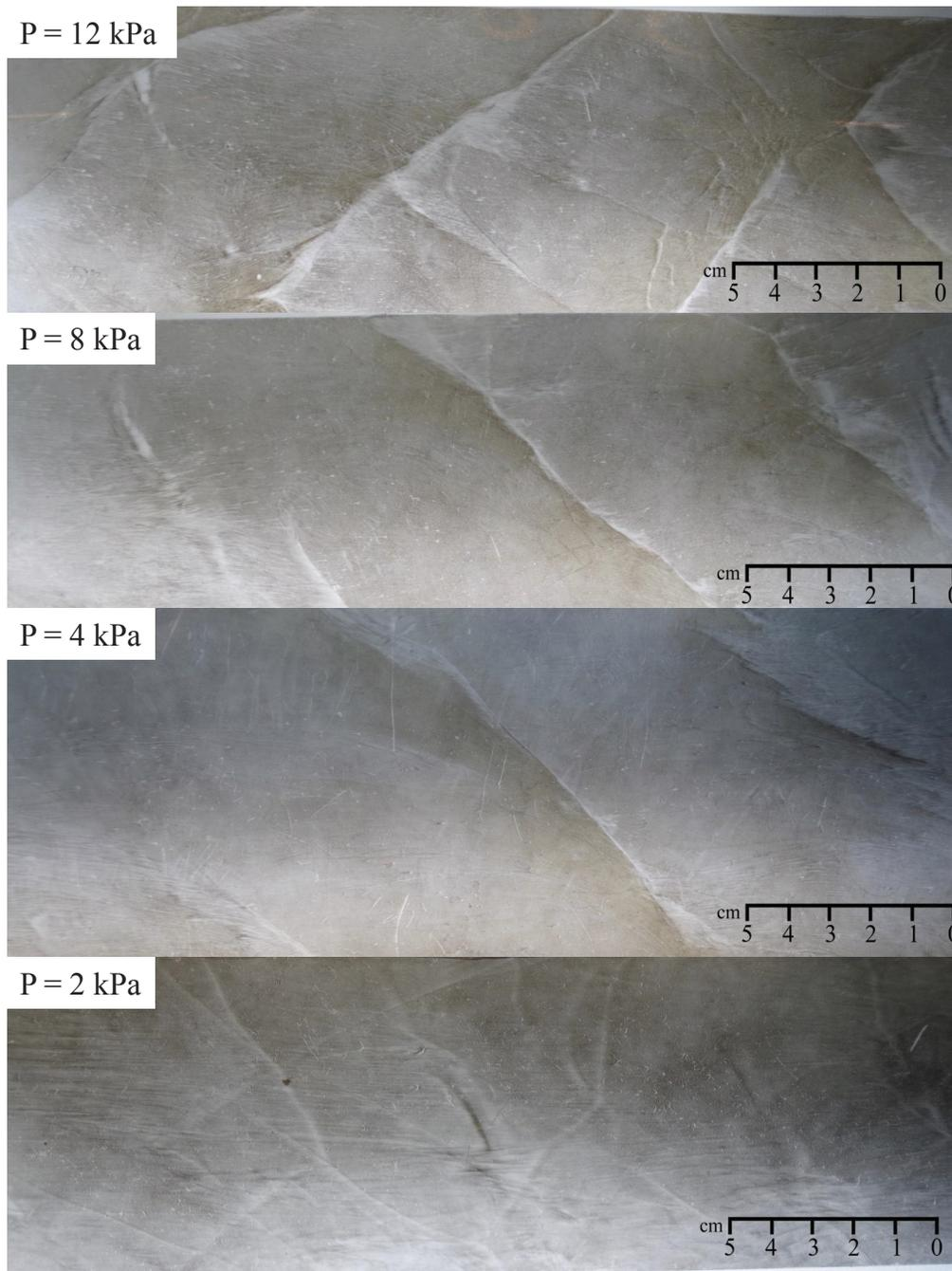
Figure 3–10: Smoked foils for  $\text{CH}_4 + 2\text{O}_2$  in the 50.8 mm diameter tube with  $\delta/D = 0.19$
