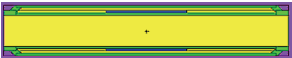
Figure 3.2 : Simulation of IBt Interseed 125 seed. Purple : water, green : titanium, blue : platinum, yellow : air.
