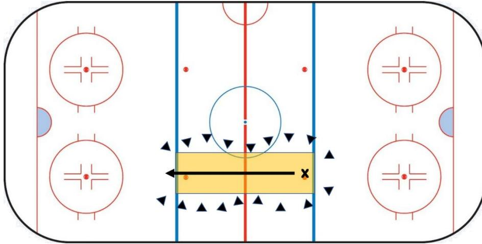
**Figure 1.** A representation of the on-ice testing set up, where motion capture cameras are represented by black triangles and an approximation of the calibrated capture area appears highlighted in yellow. “X” shows the starting position for each acceleration trial, and the arrow represents the skating trajectory of each participant.
