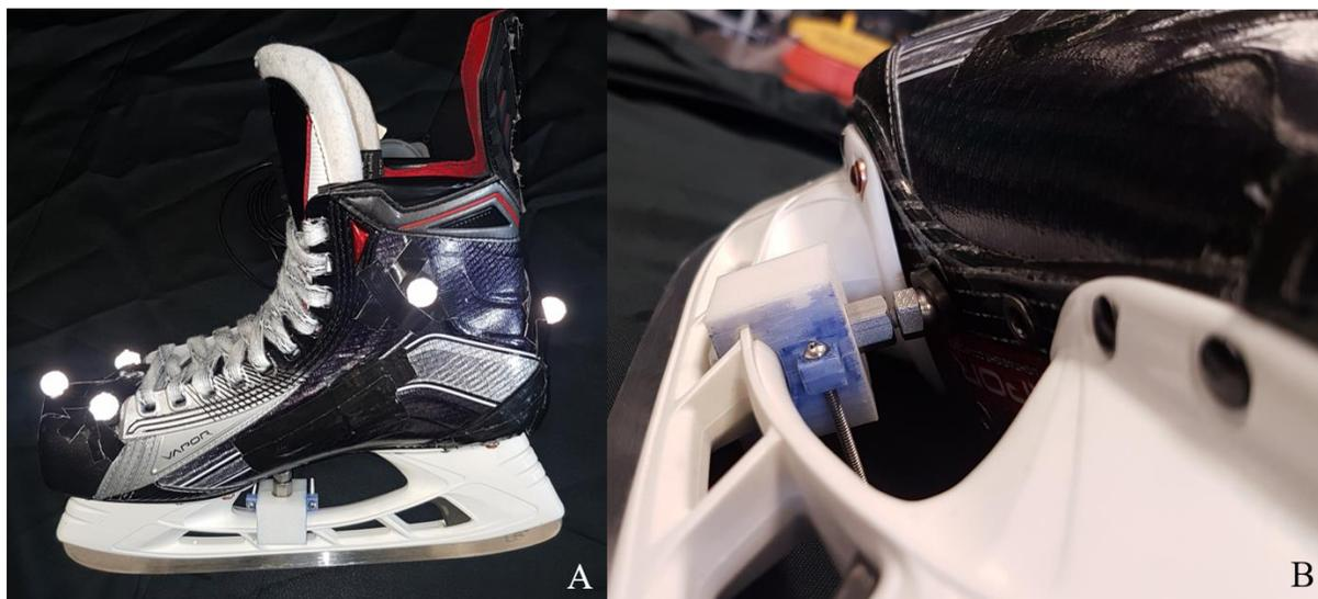
**Figure 3.** A) A skate instrumented with the force sensor and with reflective markers, B) displaying how load cells were mounted to the skate blade holder.
