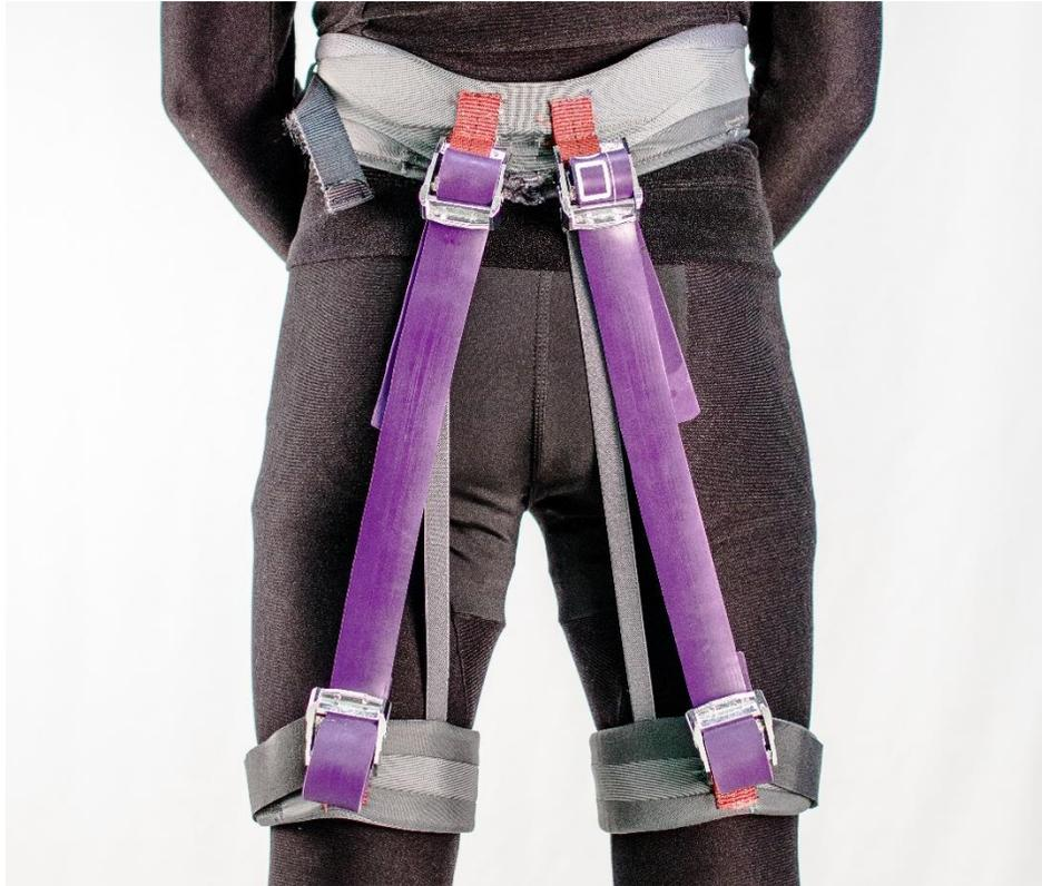
**Figure 2.** A posterior view of a participant wearing the system of elastic assistance with the “Stiff” Elastic condition
