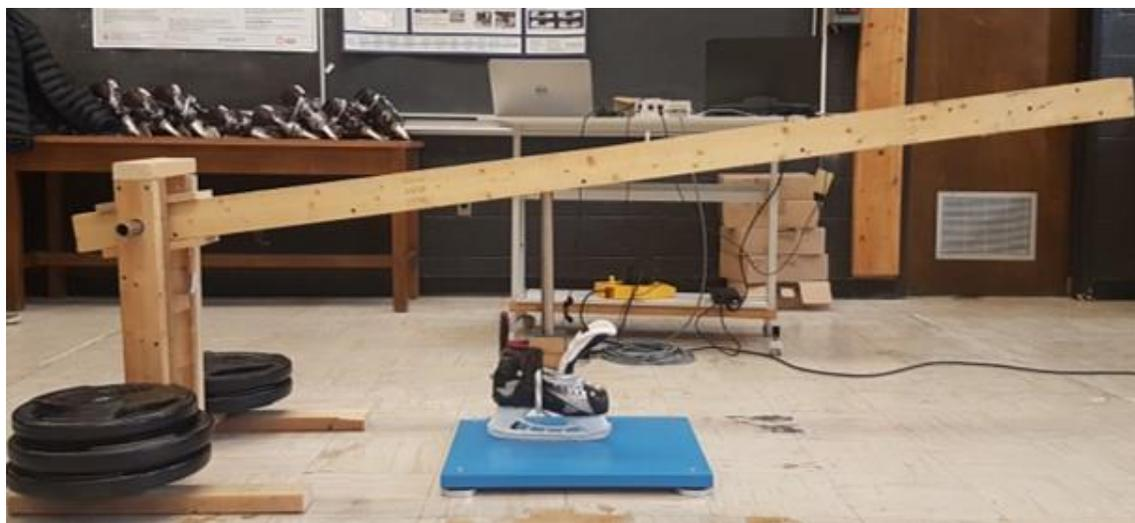
**Figure 4.** The load cell calibration apparatus
