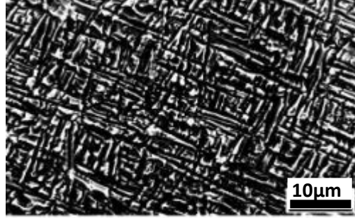
Figure 7 Ti-3.5Al-5Mo-4V microstructure after solution treatment and double aged for 2 h at 300 °C and 500 °C for 8 h (adapted from Ji et al. [31])
